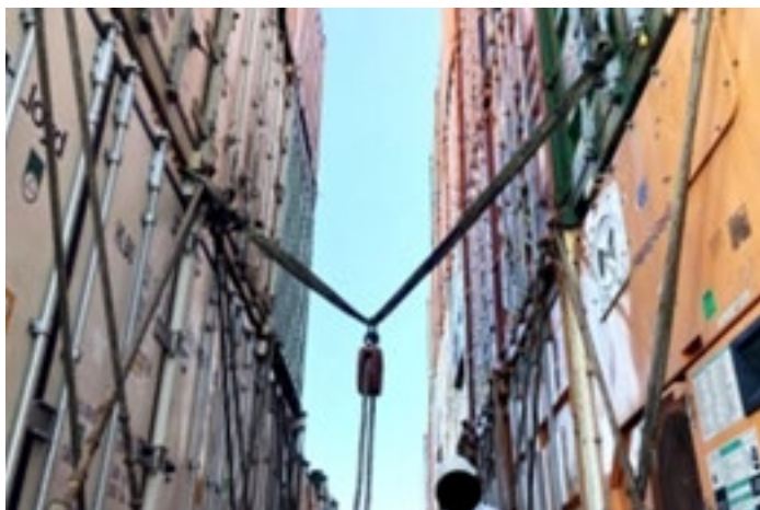
Sling construction for evacuation via the access hatch (simulated on 19/10/2021). Photo credit: BSU
