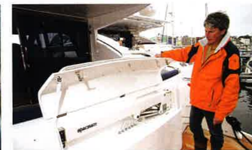
The optional tender crane is housed in the transom
