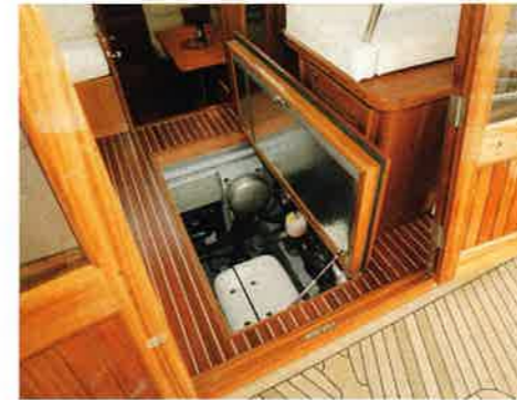
Engine access is via the cockpit or the wheelhouse
