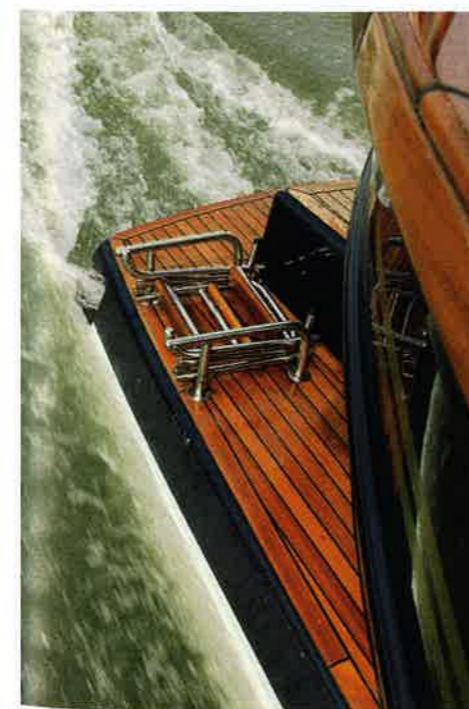
The beaver-tail bathing platform is integral to the hull
