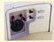
battery switches and the remote engineroom fire-extinguisher control.
