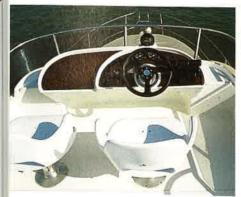
upper helm The two plastic seats are basic in design, but adjustable and quite comfortable. The console spreads itself along the front of the bridge, offering a tidy instrument display and plenty of space for additional equipment.
