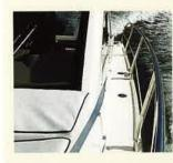
side decks Large-diameter outboard-leaning guardrails extend right aft, making the most of the 8in of deck width.
