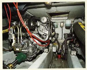
The main entrance to the engineroom is straightforward, via a hatch in the cockpit sole. But a further hatch in the saloon thoughtfully allows quick and easy access to the dipsticks and strainers.
