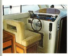
lower helm A two-tier console has standard switches laid out in a neat row, meeting up with the throttle controls to port. It includes a large space for additional electronics. Although fixed, the single bench seat is comfortable enough, and a single-piece forward screen and large side screens ensure excellent visibility.
