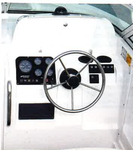
below The helm has a lockable electronics pod.
