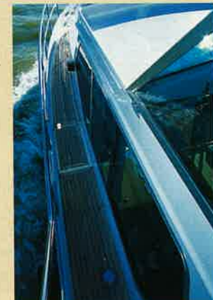
side decks Generously wide, these benefit from a high gunwale and sturdy guardrails, but no inboard handrail. Teak cladding is an optional extra.
