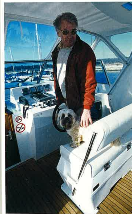
helm Centrally positioned, the simple console has smaller instrument heads ranged across in front of the skipper, and plenty of gently angled fascia for adding a radar or plotter, although no electronics come as standard. The fold-down screen is served by two sturdy wipers, and the wide single swing-back seat has just enough room for the skipper and an old sea-dog!
