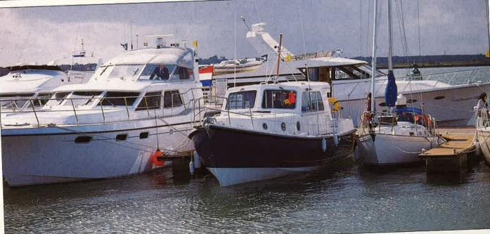
superstructure, carefully offset off by the custom-built portholes in the coachroof, allow full standing headroom throughout and a safe, deep well in the rear cockpit. A short extension to the pilothouse allows the rear door to be left open even on rainy days, and offers a landing for the optional cockpit canopy.
