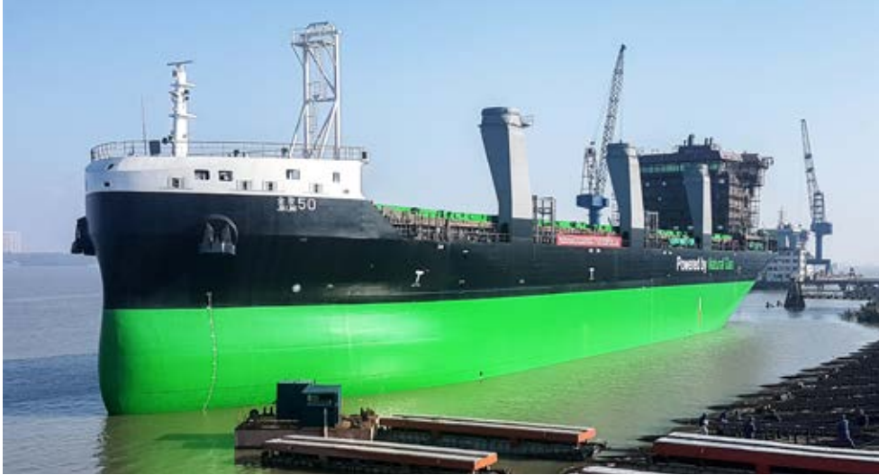
ESL Shipping's new bulk carriers Haaga (left) and Viikki are the world's first LNG-powered Handysize bulk carriers.
