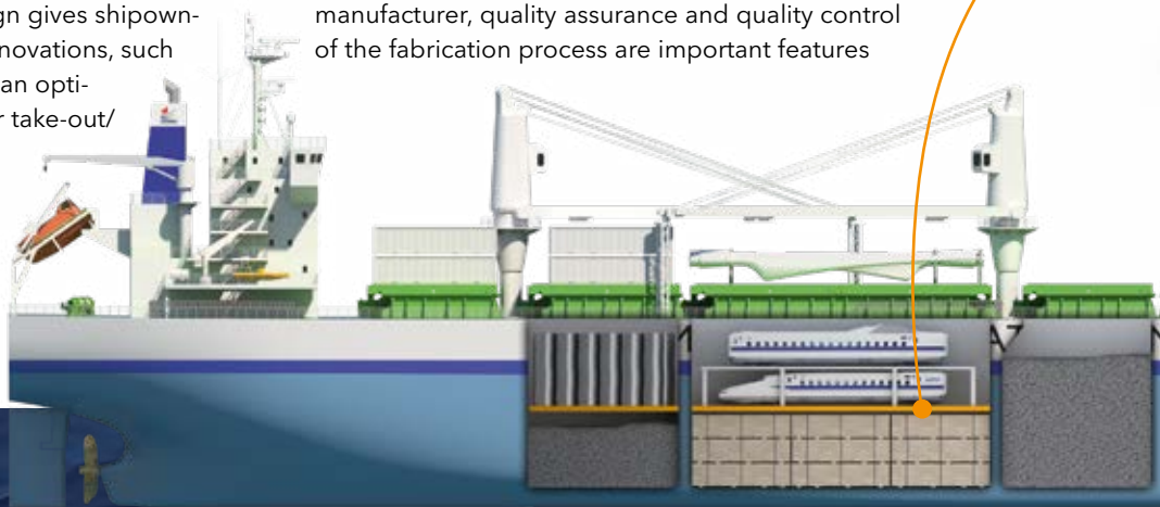
Tween decks, two elongated cargo hatches, and various alternative options make this design highly flexible.
