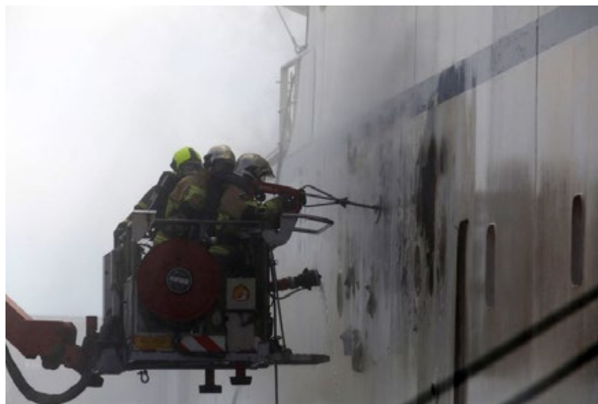
Figure 5 – Cobra Cutting Extinguisher applied by Amsterdam Amstelland Brandweer from an aerial ladder
