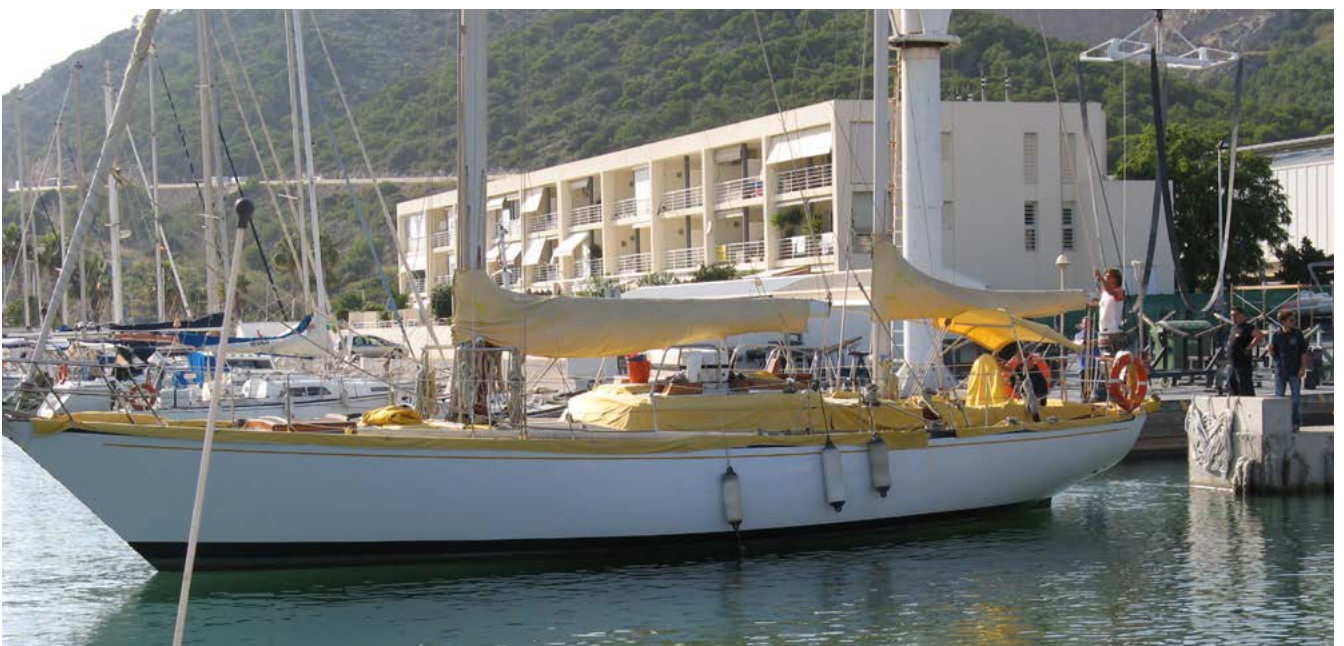
The boat below is a pre-purchase survey in Barcelona of a 50 foot German Frers designed ketch built in 1977 at the Sarmiento Shipyard in Argentina of Uruguayan Cedar planking on laminated mahogany frames.
