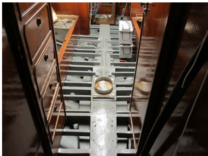
< A view of the 'I'-beam keel-girder with mast-step and recessed thru-fastened keel-bolts.
