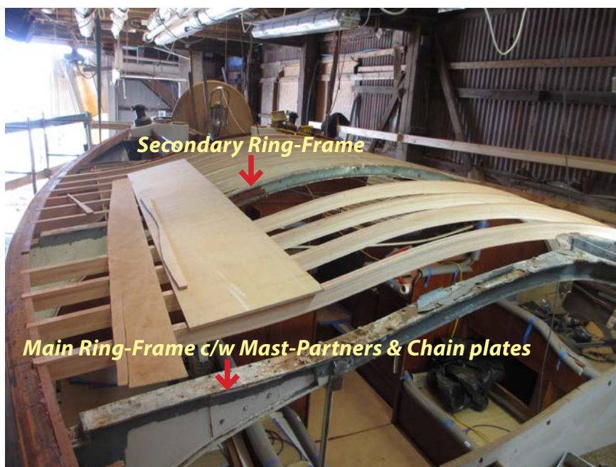
^ The new deck beams being fitted into the new beam-shelf and showing the two aluminium ring-frames.
