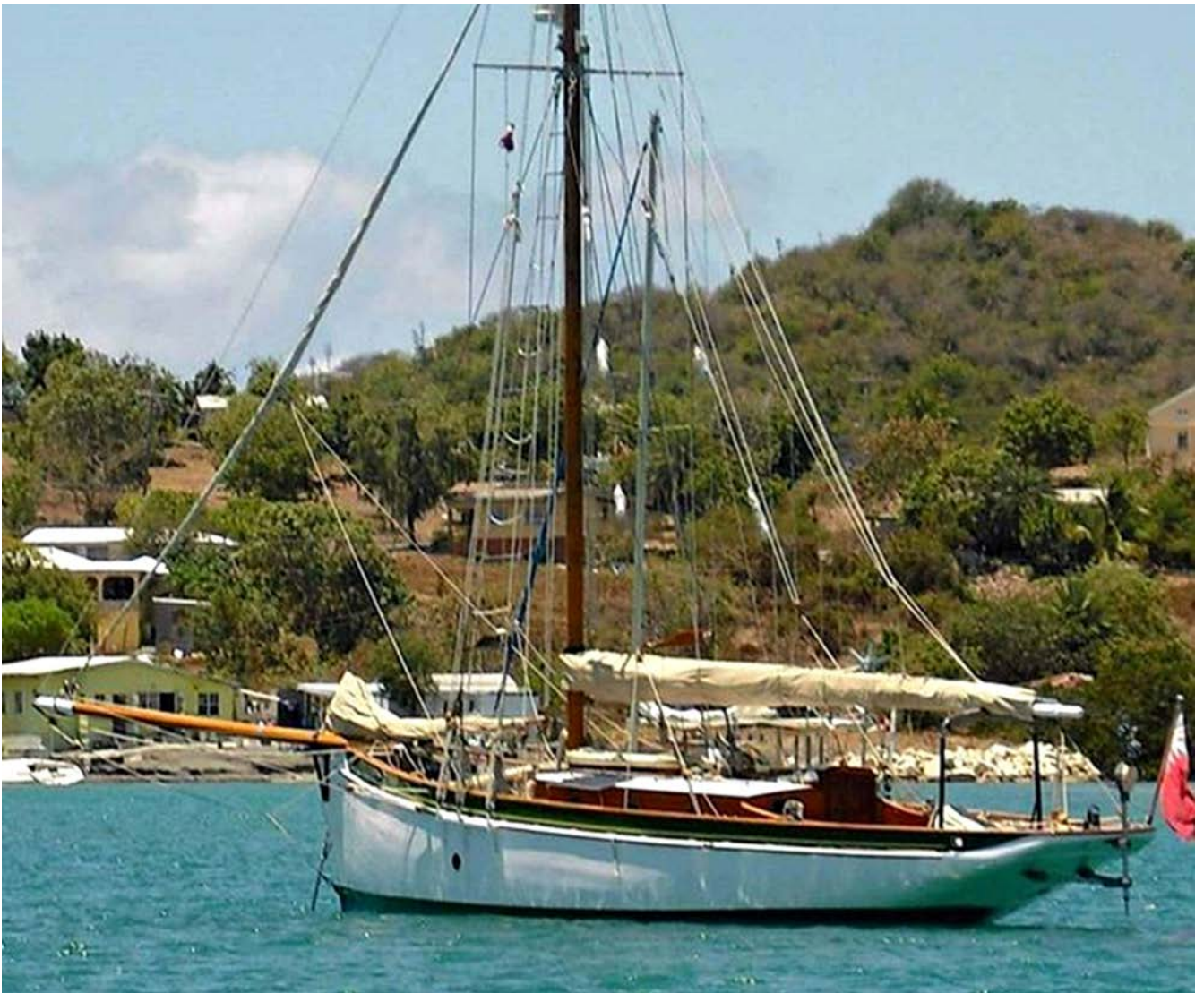
The boat above is a condition survey for insurance of the 40 foot Boston Smack 'Rhoda Gostelow' at anchor in Antigua. She was built in 1937 of Russian Red Pine on sawn-oak frames.
