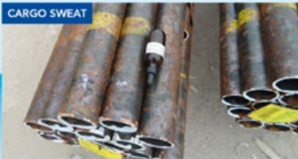
Surface corrosion or rust due to cargo sweat.
