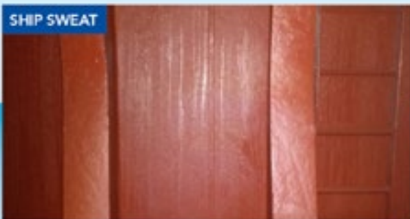
Ship sweat on the shell and side frames of the cargo hold.
