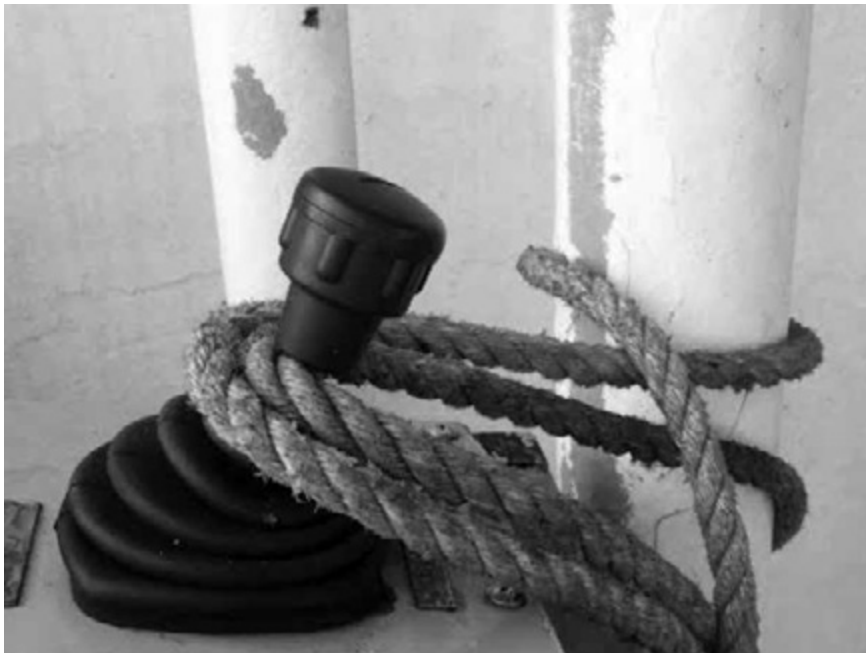
Figure 1: Winch control lever tied with a rope
