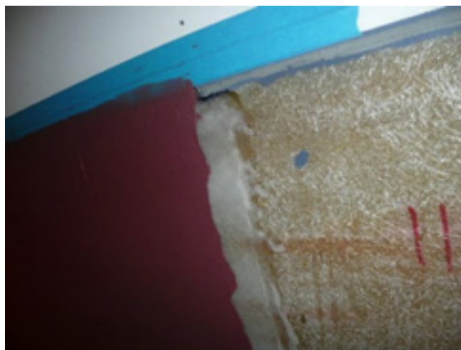
The photographs above show the previous top right blistered hull when peeled and the layers of repair, the void within the laminate has been filled and the hull prepared and laminated with glass cloth prior to fairing and then re-gel coating.
