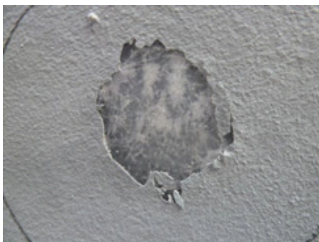
No Osmosis here, dry laminate left, where there has been little or no wetting out of the CSM (Chopped Strand Mat), fibres and on the right wicking where moisture has travelled by capillary action through the hollow underlying dry glass fibres causing them to swell, turning white.
