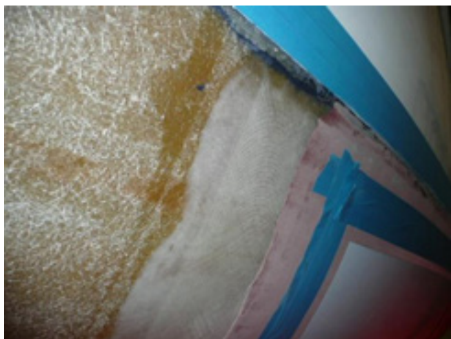
The photographs above show the previous top right blistered hull when peeled and the layers of repair, the void within the laminate has been filled and the hull prepared and laminated with glass cloth prior to fairing and then re-gel coating.
