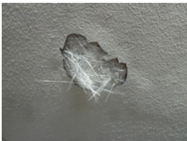
No Osmosis here, dry laminate left, where there has been little or no wetting out of the CSM (Chopped Strand Mat), fibres and on the right wicking where moisture has travelled by capillary action through the hollow underlying dry glass fibres causing them to swell, turning white.
