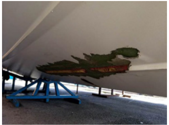
No Osmosis here either, this is delamination as a result of poor wetting out and consequently a lack of bonding between the layers of laminate in the hull of a brand new motor yacht straight from the factory; just because it is a new boat with a dry hull does not mean that it does not have an underlying problem.
