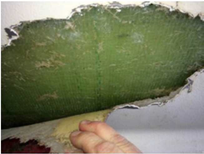
No Osmosis here either, this is delamination as a result of poor wetting out and consequently a lack of bonding between the layers of laminate in the hull of a brand new motor yacht straight from the factory; just because it is a new boat with a dry hull does not mean that it does not have an underlying problem.
