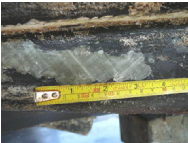
Above left a 95 foot motor yacht with underwater hull modifications, which had not been gelled, with the underlying mat strands clearly visible. Above right with the outer skin removed the damage of water ingress into this foam core can be clearly seen, local moisture readings and hammer soundings identified the presence of this defect.
