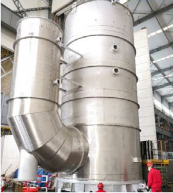
Figure 3: Open-loop marine scrubber manufactured by ContiOcean Environment Tech Co., Ltd in super duplex stainless steel
