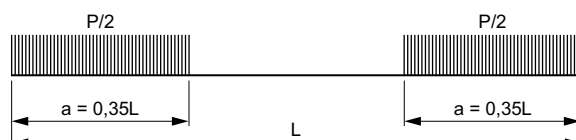
Figure 3 : Vessel weight distribution - Hull girder load case 2
