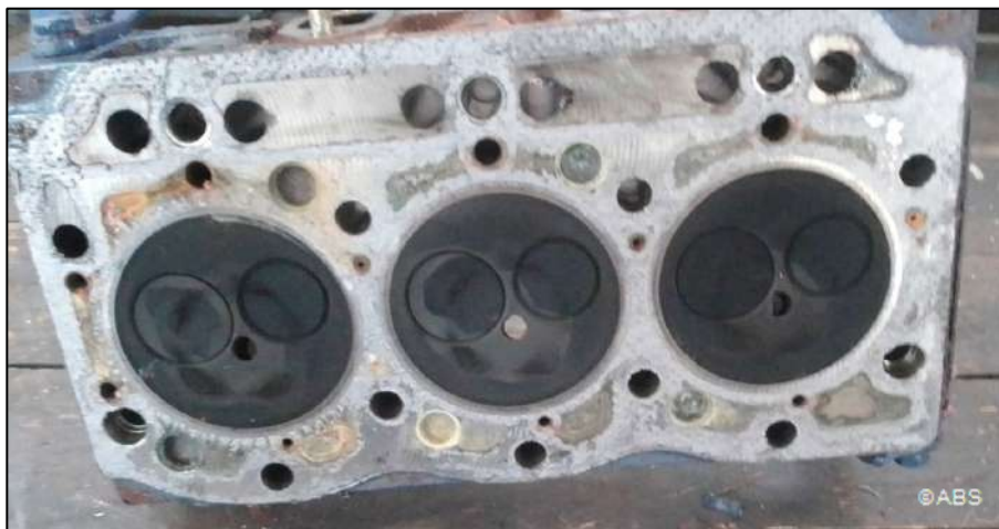
Inoperative freefall lifeboat engine/unit dismantled for overhaul
