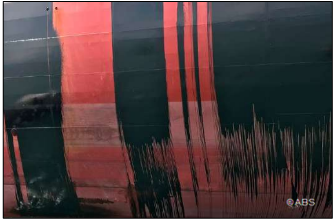
Oil spill on deck and over the side due to bunkering procedure not followed
