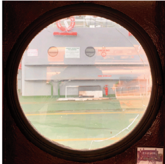
Flame Front extended aft to crack the Port-Light Glass
