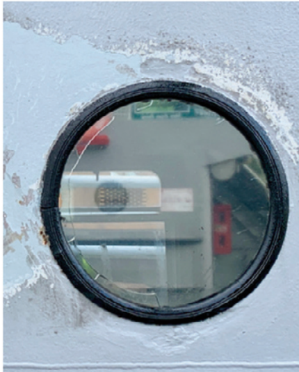
Flame Front extended aft to crack the Port-Light Glass
