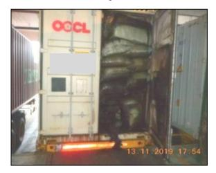
Figure 5: Right rear door open, showing burnt bags
