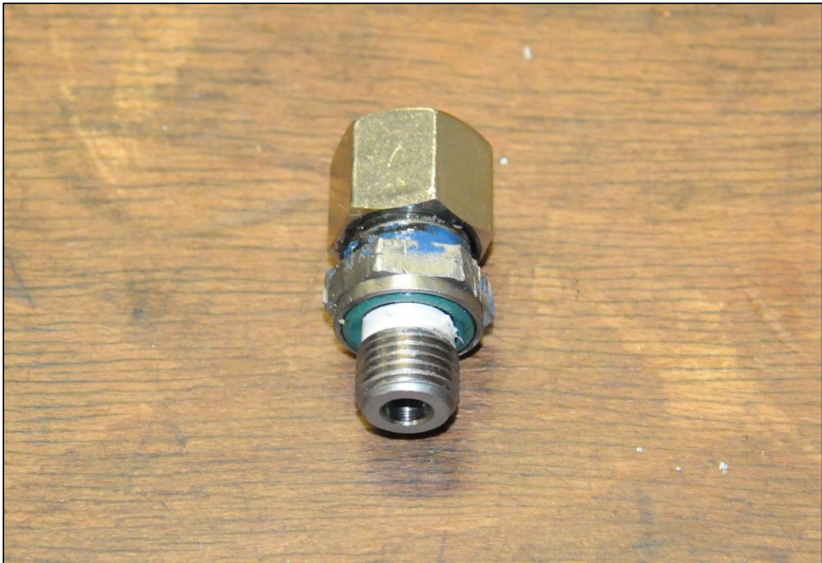
Figure 11: Double nipple Ermeto L10 with cap nut
