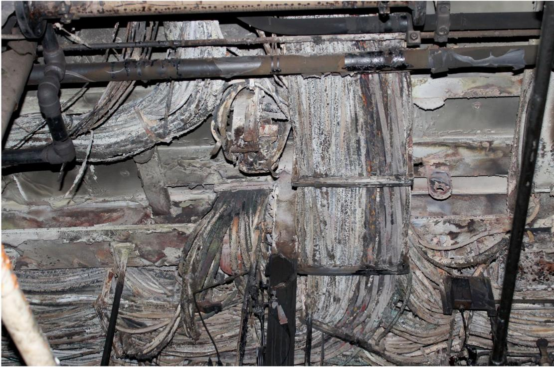
Figure 11. Engine control room consoles, showing fire damage (Source: TSB)
