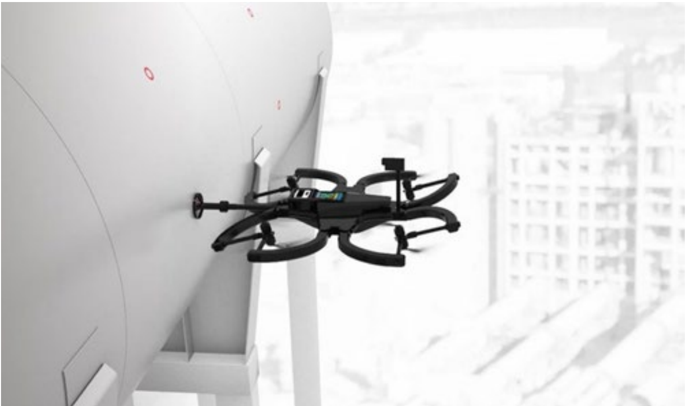
Above: The "Skygauge" UT which combines a UAV (multi directional rotors for greater accuracy and directional control) with an ultra-sonic probe and an inbuilt LIDAR to allow for accurate positioning and distance measuring from the host material.
