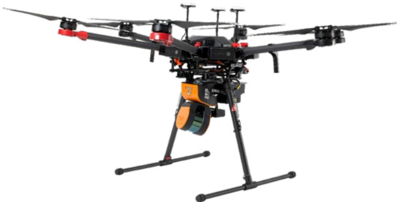
Above: A multi rotor UAV fitted with a GeoSLAM LIDAR System.
