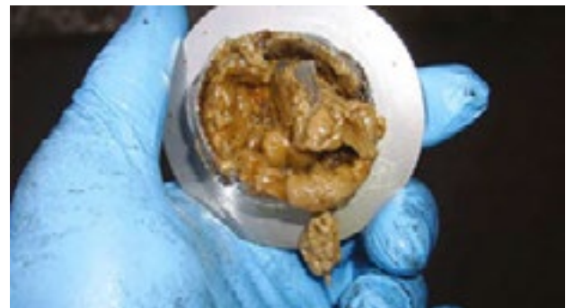
Figure: Fuel filter clogged with diesel bugs
