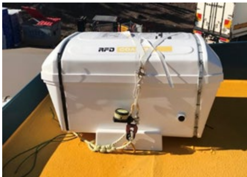
Correctly fitted HRU on a life raft
