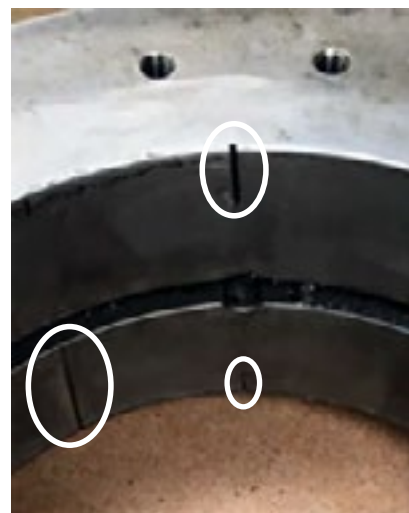
Figure 1: Bearing housing notches from disc cutter
