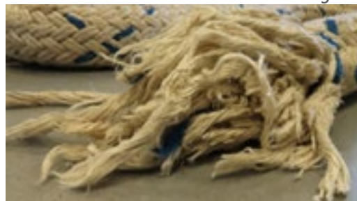
A parted mooring line
