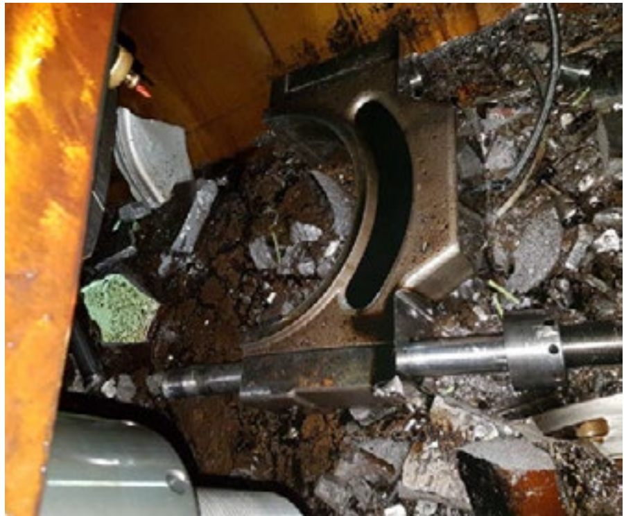
Figure 2: Post-failure engine component debris in sump
