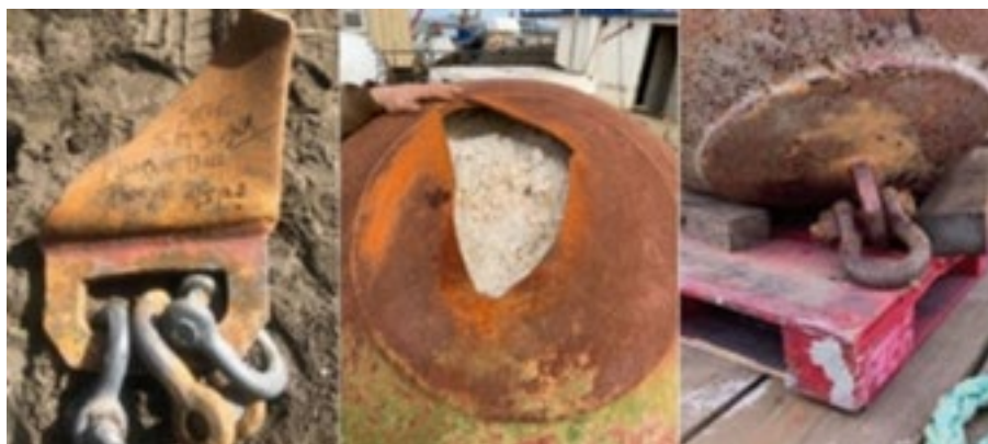
SM-3 mooring buoy: failed padeye (with three shackles) that separated from buoy (left), damaged top with padeye missing (center), and undamaged bottom padeye (right). (Source: Alaska Marine Surveyors and Northline Seafoods).
