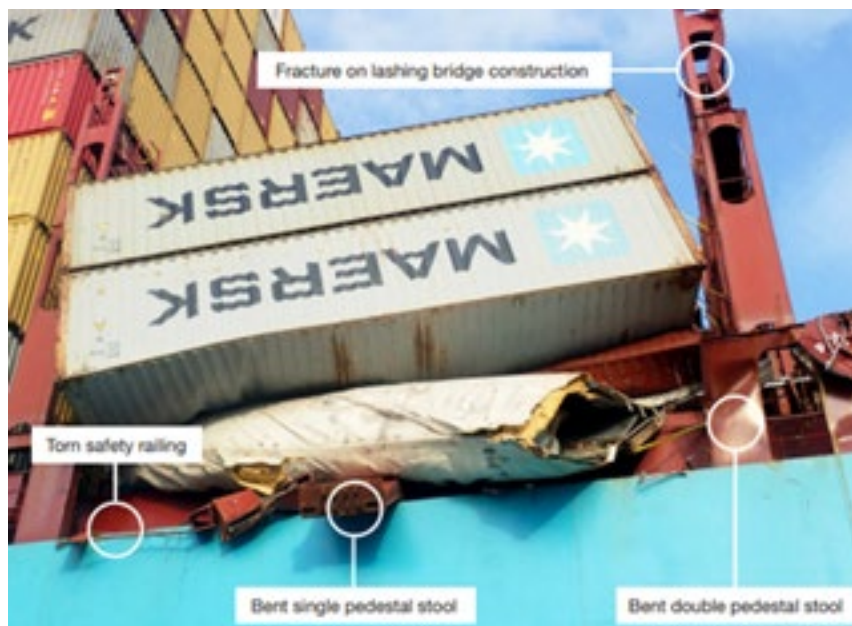
Parametric rolling is the suspected cause of the loss of containers from Maersk Essen. Photo credit: DMAIB
