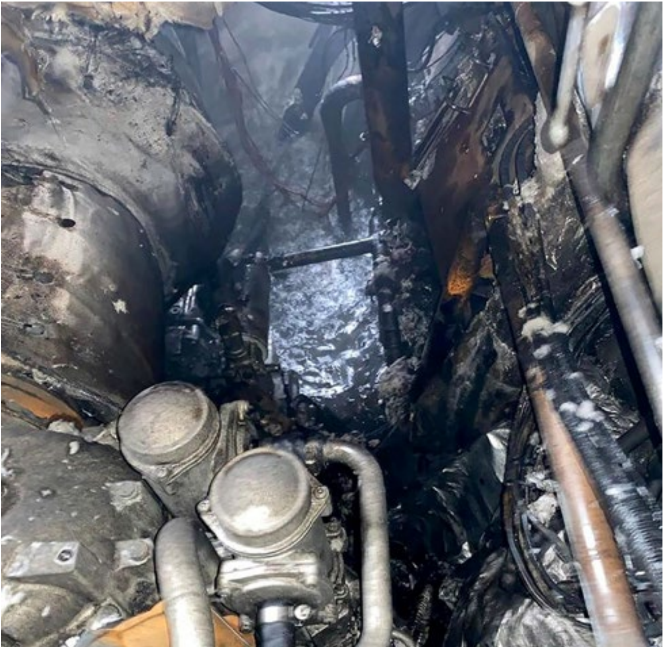
Figure 3: Fire damage in the engine compartment
