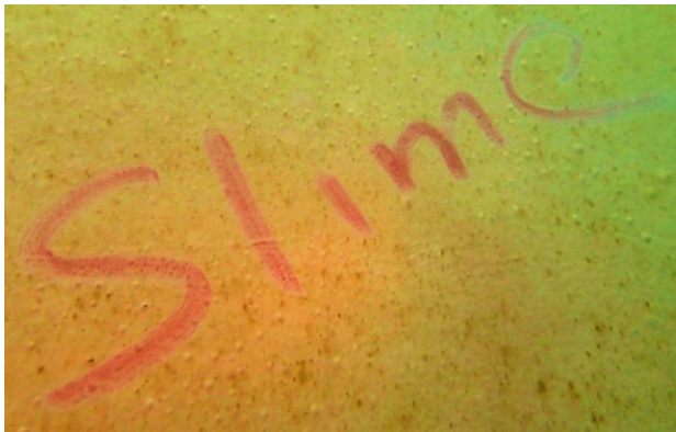
Slime layer on the surface of a hull
