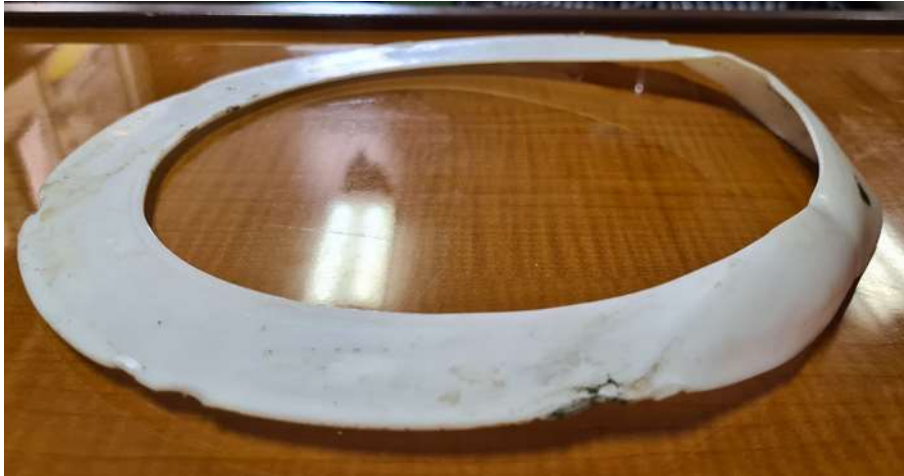
Figure 9 - Damaged gasket after disassembly
