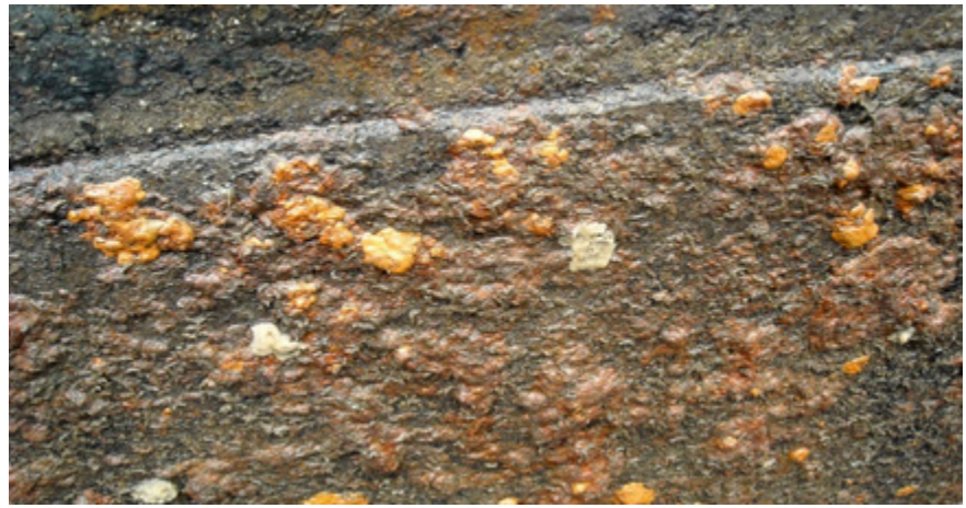
Photograph 2 - Extensive Gallionella Ferruginea attack on a Narrowboat
