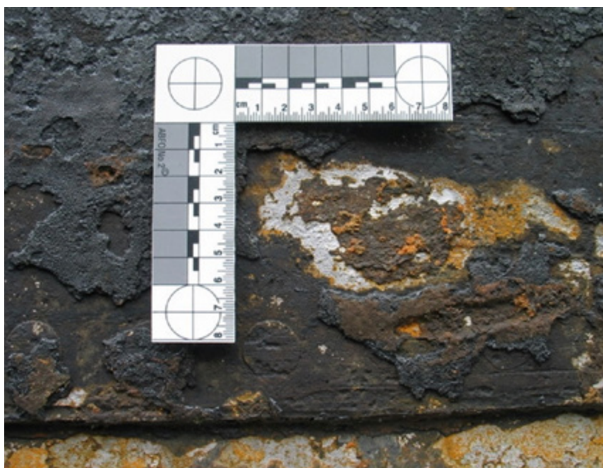
Photograph 1 - Attack on a Steel Narrowboat by Microbes of the Genus Thiobacillus
