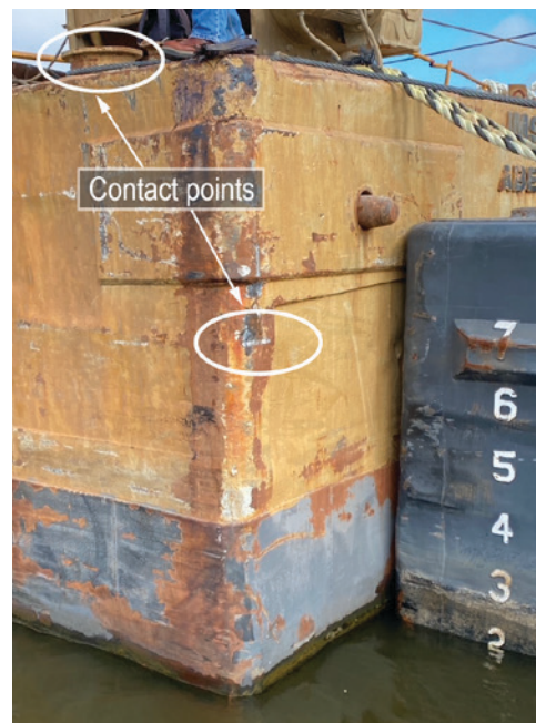
Figure 84. Left: Simple representation of fendering and swing span lighting; profile (top) and plan (bottom) views. BACKGROUND SOURCE: COAST GUARD. Middle and Right: Postaccident damage to the corner of barge JMSS Mobile , with damage markings and scrapes about 6 feet above the waterline, and to the northeast corner of the Barataria Bridge, with points of contact with the barge JMSS Mobile indicated. SOURCE: ANONYMOUS.
