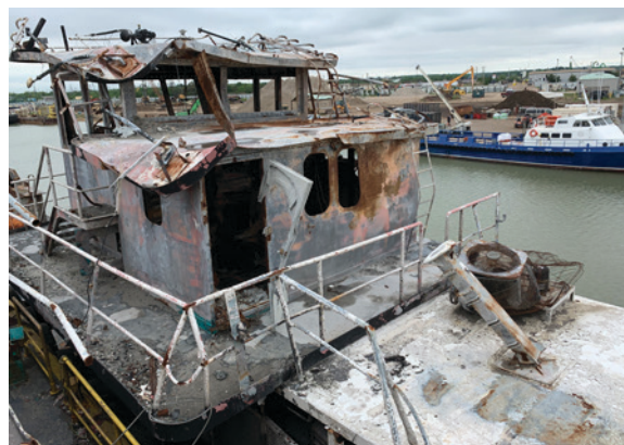
Figure 138. Post-salvage images of the Waymon Boyd lever room and captain's office ( above ) and engine room portside bulkhead, bowed outward ( right ).
