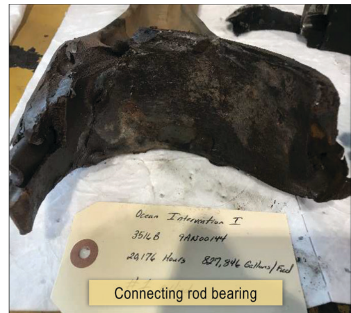
Figure 117. The yellow bracket identifies the damaged area of the main crankshaft of the no. 3 DG (left), where the no. 1 connecting rod bearing failed (right). SOURCE: OCEANEERING INTERNATIONAL, INC.
