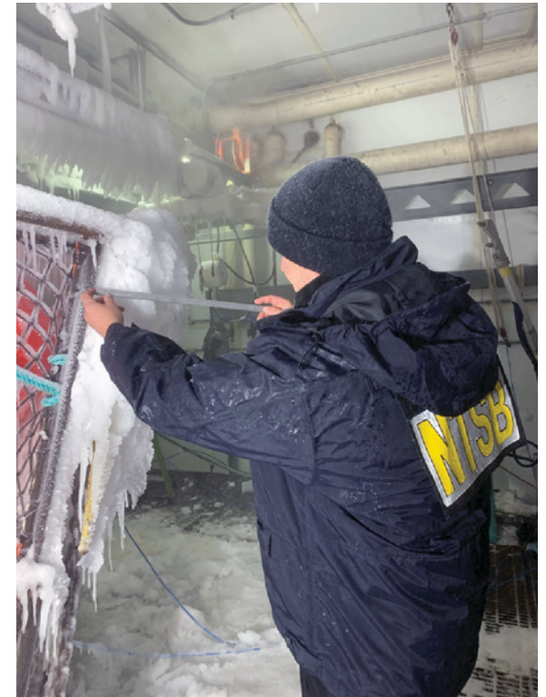
Figure 161. An NTSB investigator measures ice accretion on a crab pot during the Scandies Rose investigation.
