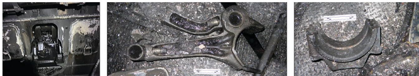
Figure 93. Holed crankcase at no. 4 left cylinder inspection cover (left), no. 4 left and no. 4 right connecting rods (middle), and connecting rod clamp (right).
