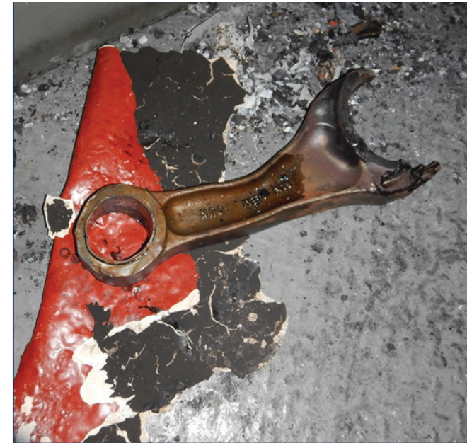
Figure 115. The damaged section of the engine (left), as indicated by the yellow square, from where the connecting rod from the no. 3 DG (right) was ejected. SOURCE: OCEANEERING INTERNATIONAL, INC.; COAST GUARD
