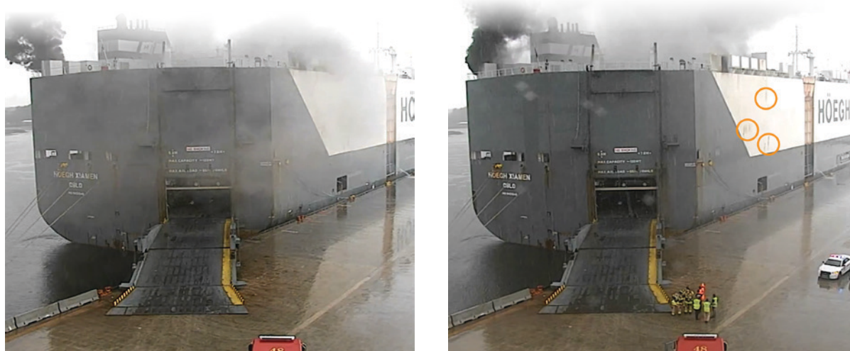
Figure 100. Left: Engine 48 arriving on scene about 1603. Starboard vents 10/11E and 7/8E and port vents 10/11E and 9E exhibit smoke flow. Right: About 1608, 5 minutes after Engine 48's arrival, the white paint on the starboard side of the vessel exhibits thermal discoloration (circled in orange). Starboard vents 10/11E and 7/8E and port vents 10/11E and 9E exhibit smoke flow. SOURCE: JACKSONVILLE PORT AUTHORITY
