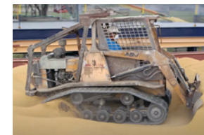
Figure 61. ZGC-owned and -operated payloader leveling off a cargo hold. SOURCE: ZGC
