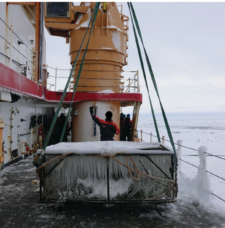
Figure 17. Crewmembers aboard Coast Guard Cutter Polar Star weigh a crab pot following a 3-day freezing spray experiment. SOURCE: COAST GUARD
