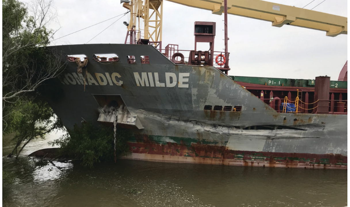
Figure 41. Nomadic Milde on the right descending bank at the Cornerstone Dock showing a gash in the hull aft of the port anchor pocket. SOURCE: COAST GUARD
