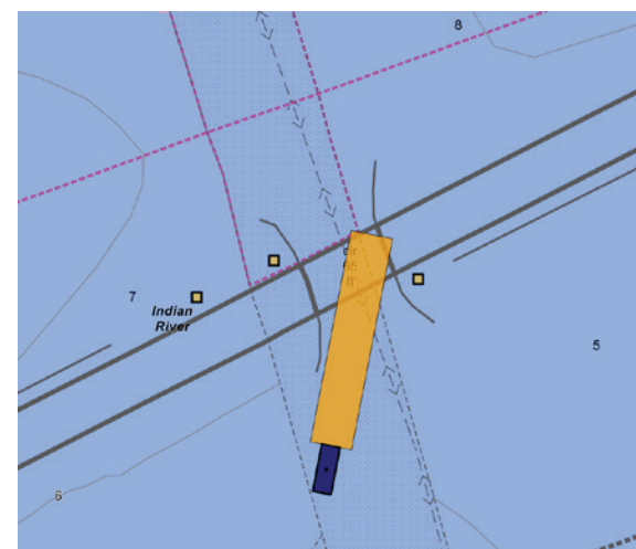
Figure 76. The approximate position of the tow after striking the protective fendering system under the Peter P. Cobb Memorial Bridge.
