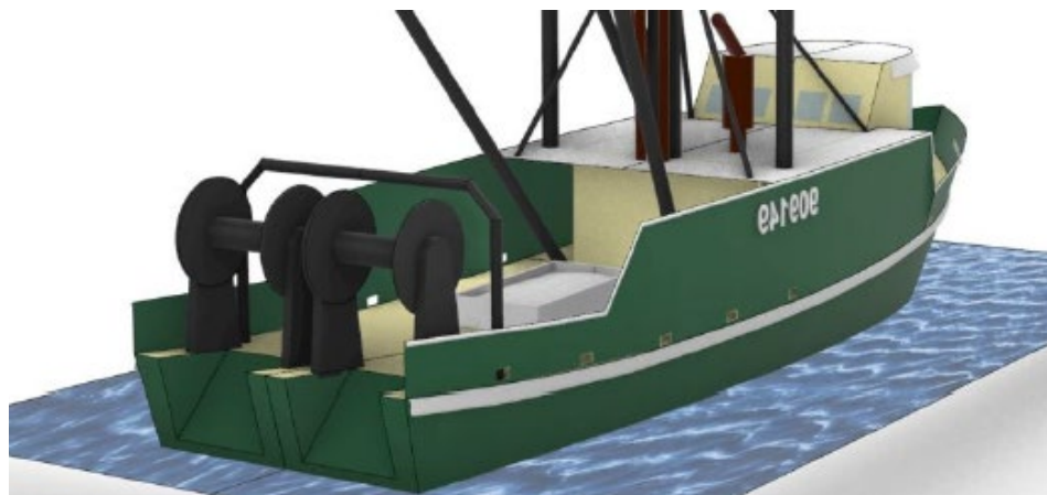
Figure 17. MSC model of Emmy Rose's starboard quarter showing aft bulwarks and stern ramps (storm gates not shown). (Source: MSC)
