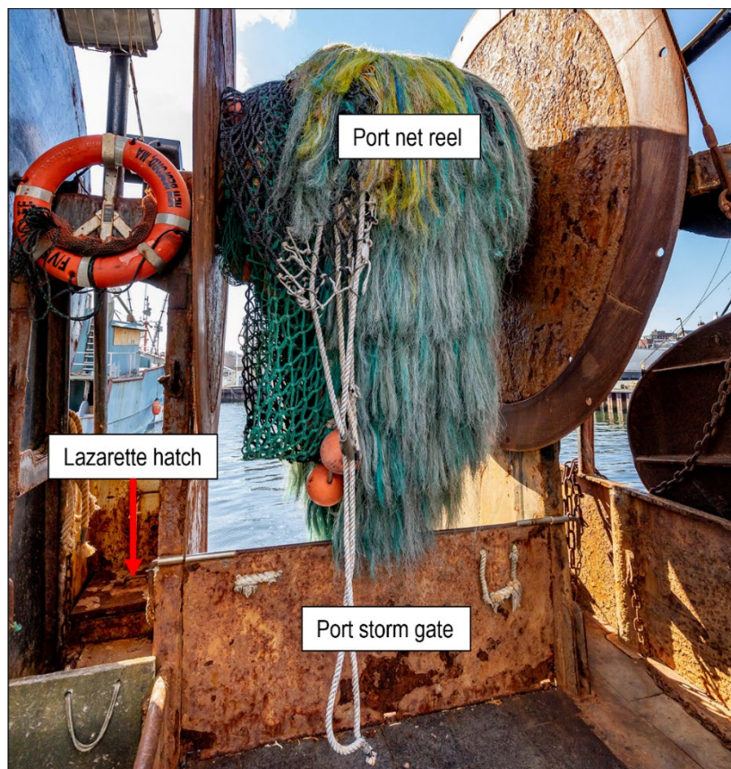
Figure 11. Port net reel, storm gate, and lazarette hatch of Sasha Lee in 2019 before its purchase by Boat Aaron & Melissa. (Background source: Blue Harvest Fisheries)
