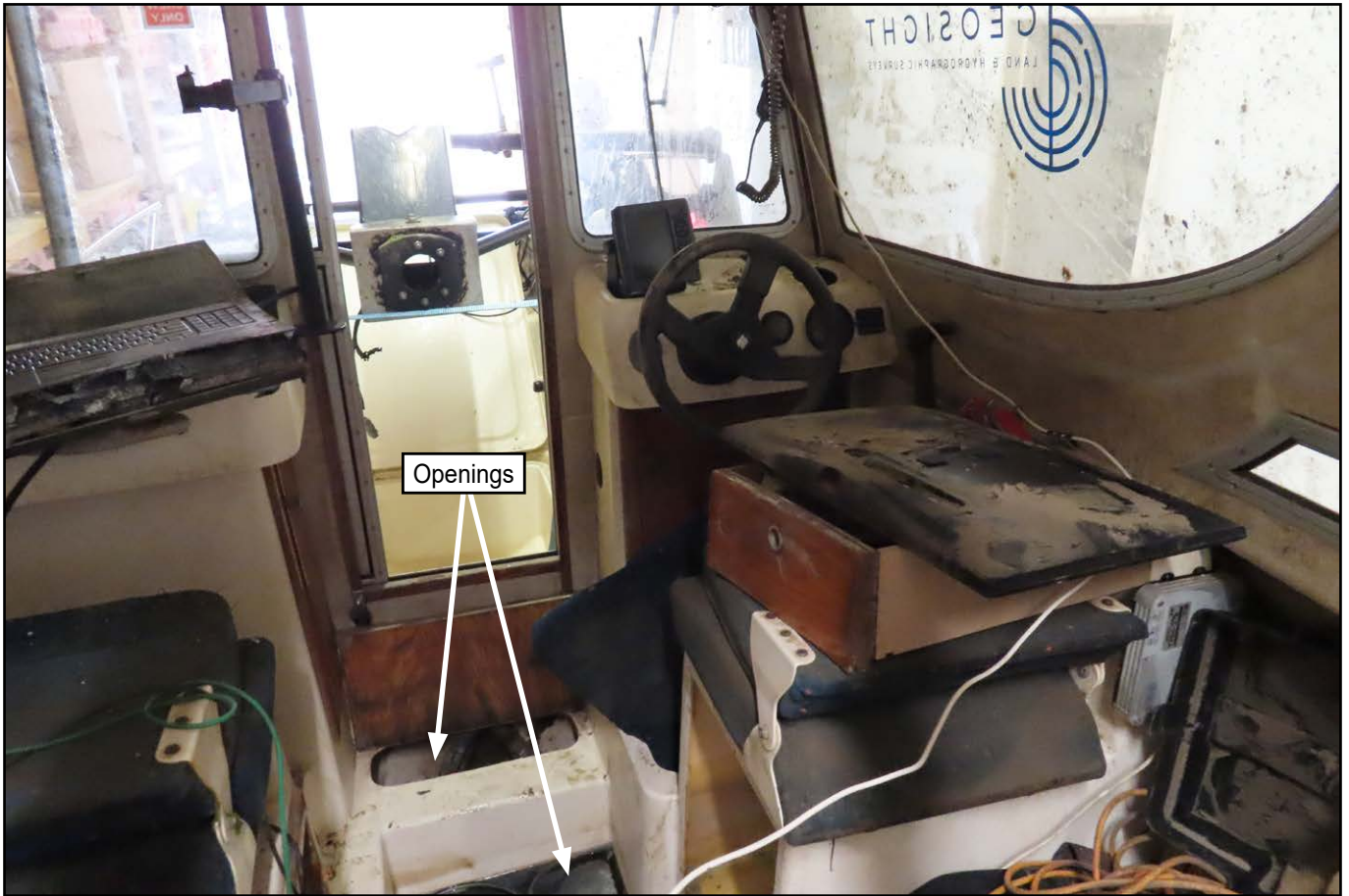
Figure 4: Bella's wheelhouse, showing openings into the void between the deck and hull mouldings
