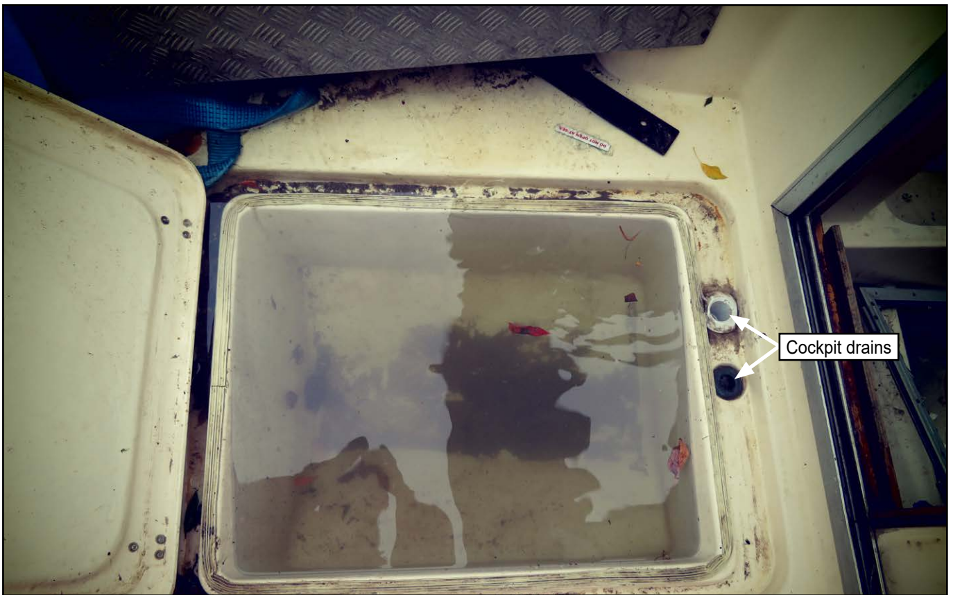
Figure 5: Forward sole locker full of water, and cockpit drains
