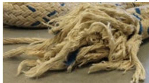
A parted mooring line
