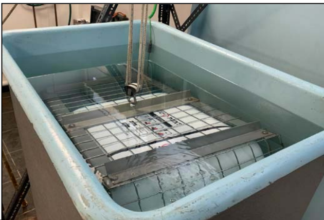
Fig.5. Waypoint Liferaft – New Sample. Serial No. W21D076 submerged in buoyancy tank (marked side up).
