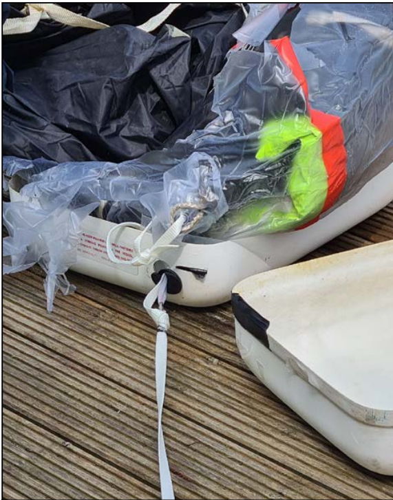
Fig.7. Waypoint Liferaft – Recovered. Serial No. W16L300 following activation. Note the grommet not released with painter line loop handle.
