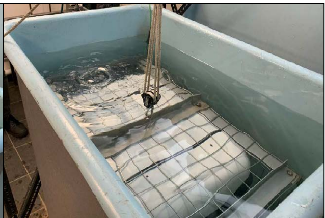
Fig.6. Waypoint Liferaft – New Sample. Serial No. W21D076 submerged in buoyancy tank (marked side down).
