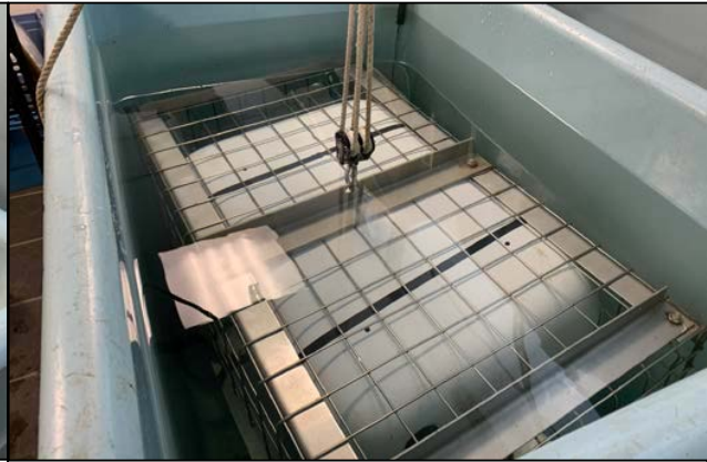
Fig.4. Waypoint Liferaft – Recovered. Serial No. W16L300, submerged in buoyancy tank (marked side down).
