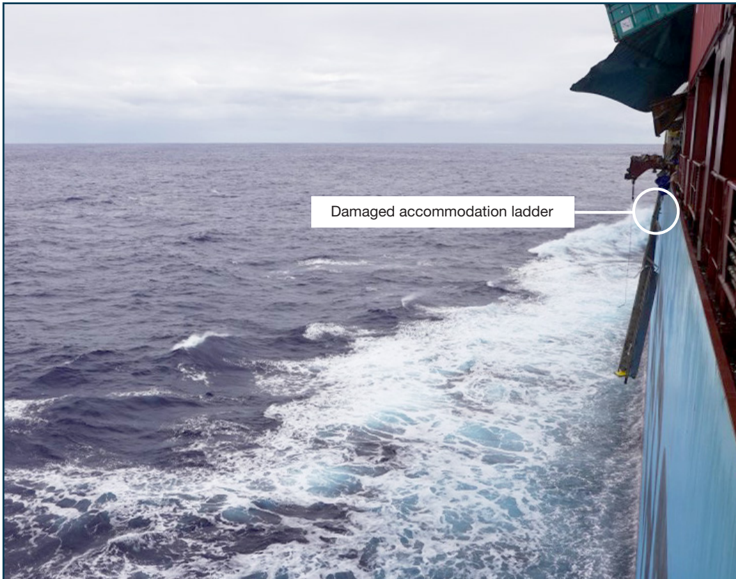
Figure 10: Damage to port side accommodation ladder Source: Maersk A/S, modified by DMAIB
