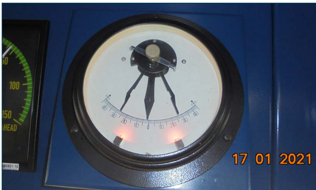
Figure 19: Inclinometer after the heavy rolling occurrence on 16 January 2021
