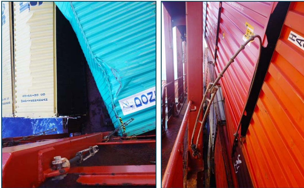
Figure 47 and 48: Example of detached and bent lashings (bay 66 and 54) Source: Maersk A/S
