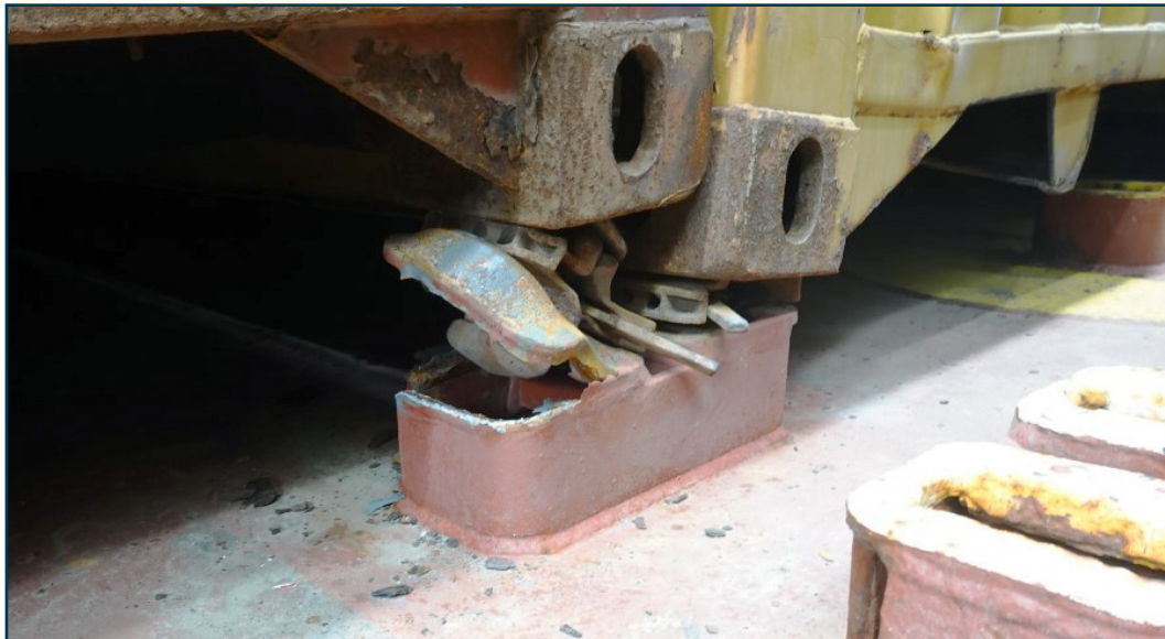
Figure 51: Example of twistlock in open position, though socket and twistlock are broken. Source: Maersk A/S
