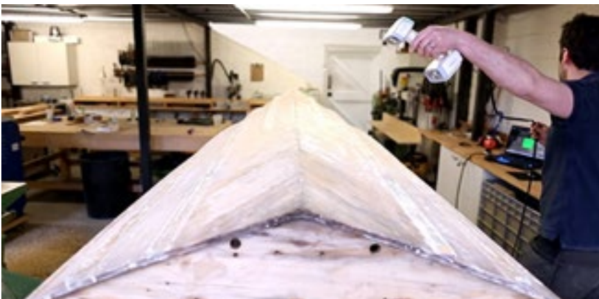
Daniel is scanning the full hull of the Stapley ski race boat in his workshop
