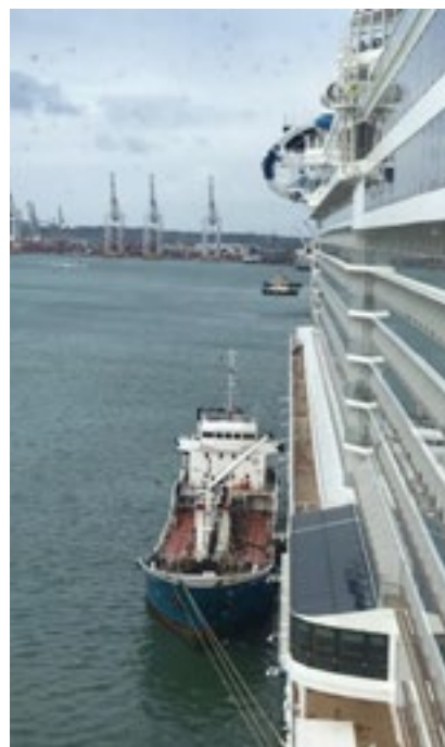
Bunker in progress
