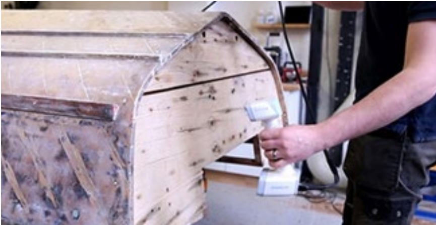
3D capturing the hull of a boat with the EinScan H hybrid light 3D scanner
