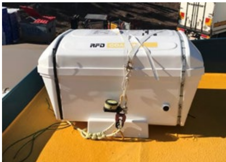
Correctly fitted HRU on a life raft
