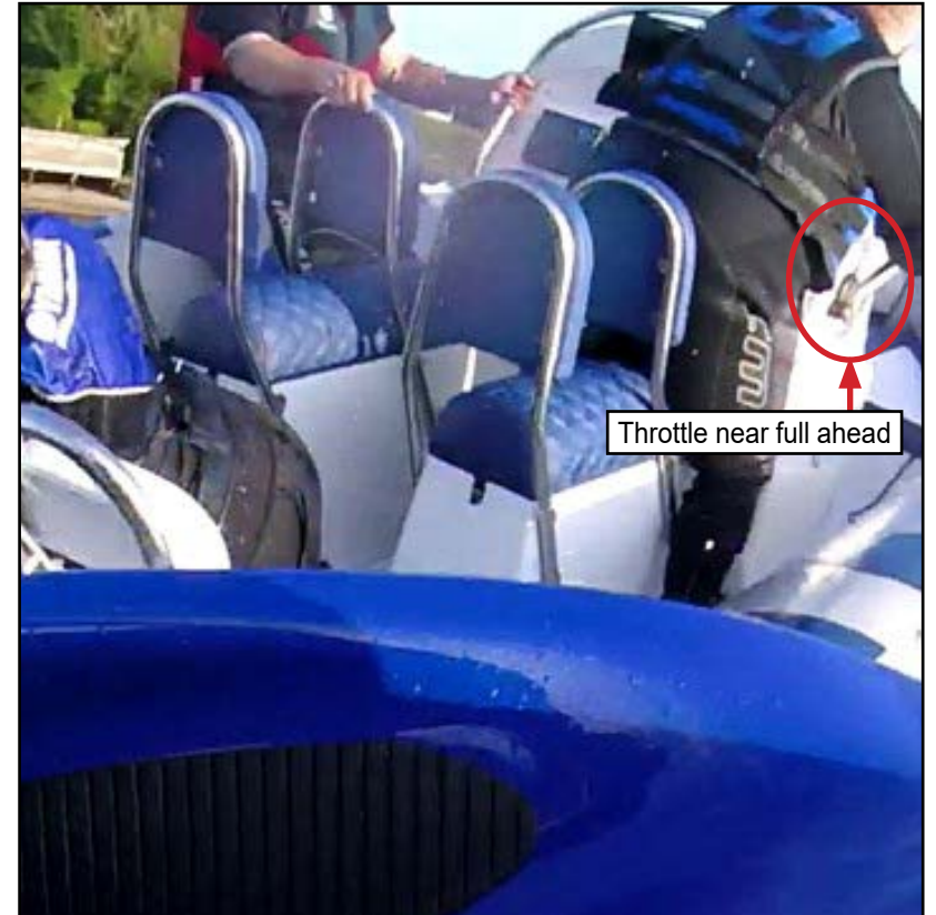
Figure 6: Rib Tickler helm console, showing the relative throttle positions for neutral and nearly full ahead
