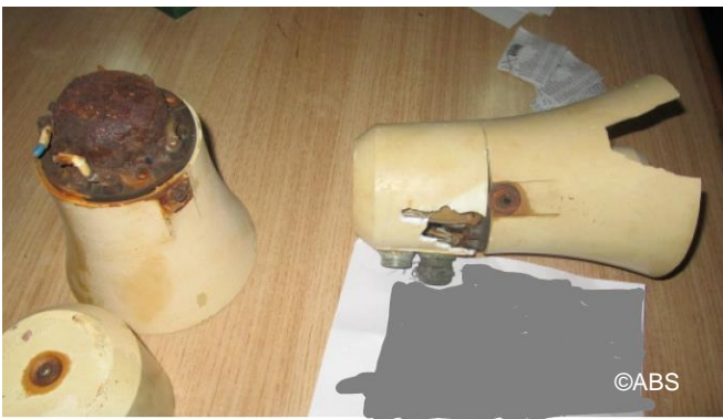
Public address system speakers damaged
