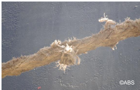
Mooring rope with broken strands
