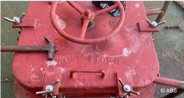
Watertight booby hatch with new dog bolts
