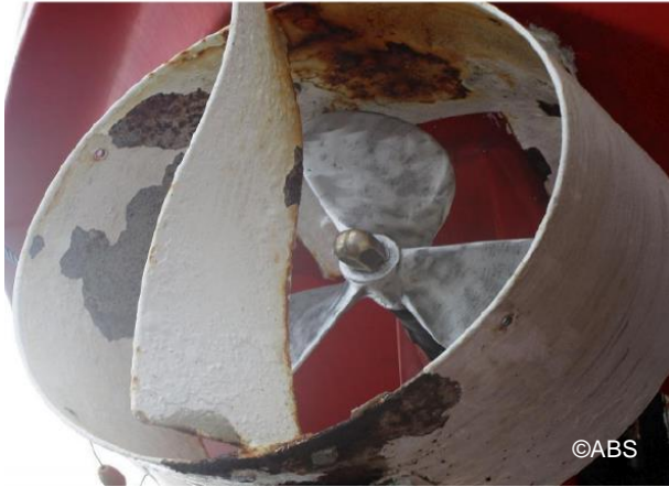
Lifeboat rudder corroded - before
