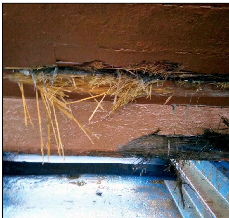
Figure 2: Damage to keel and hull planking
