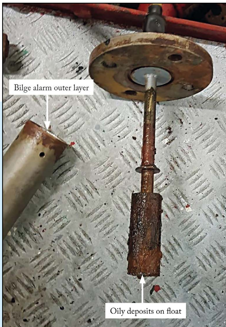
Figure 2: The disassembled bilge alarm, showing the build up of oily deposits on the float
