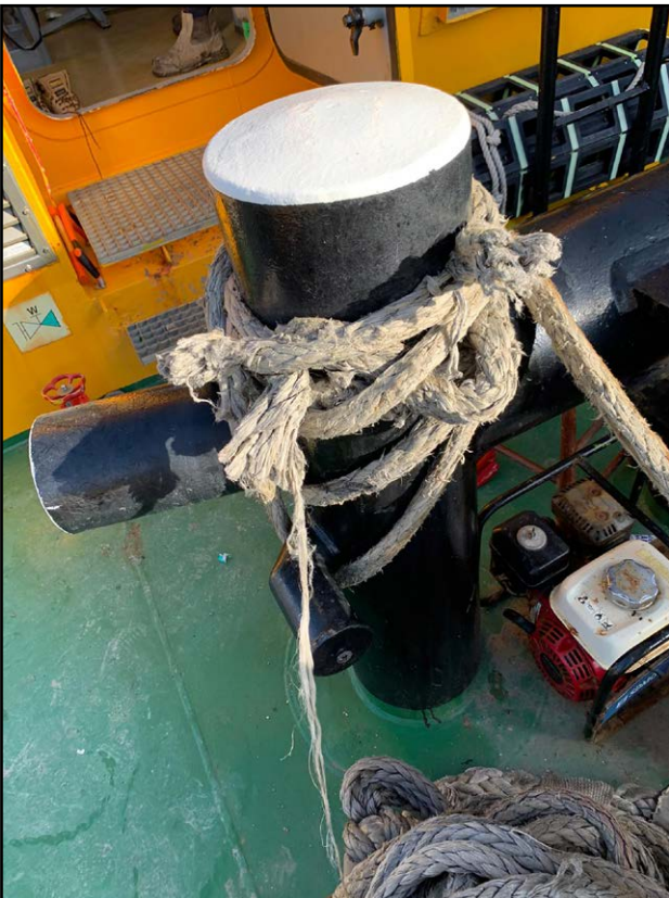
Figure 2: H post, showing cut line
