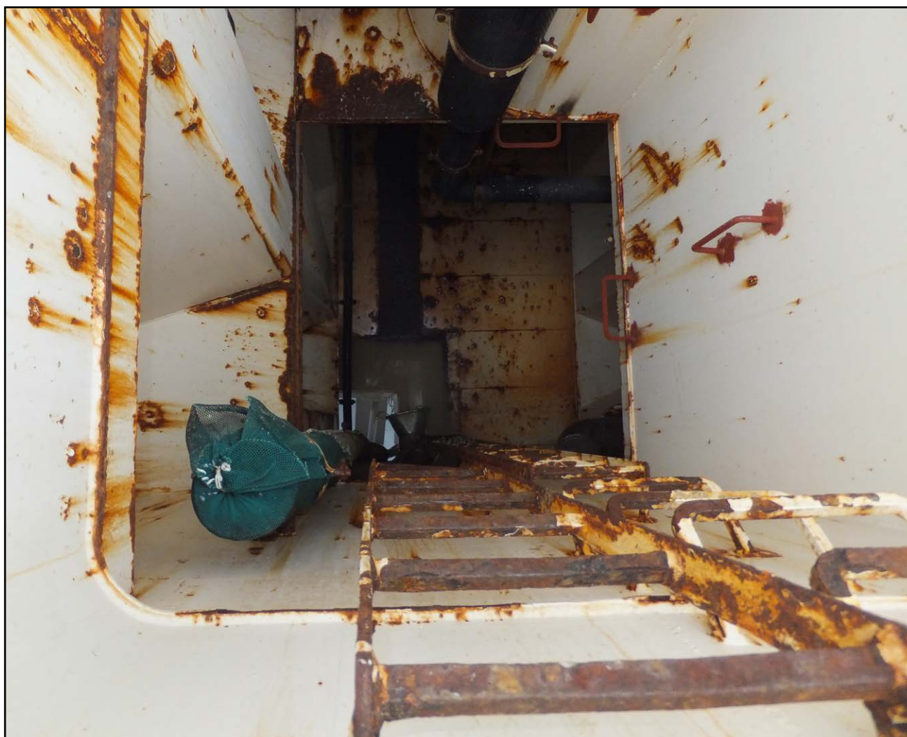
Figure 2: The view down through the access hatch into a pelagic fishing vessel's RSW tank
