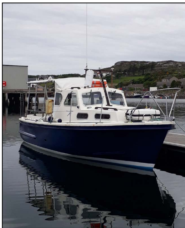
Figure: The fishing vessel before the accident, showing the liferaft on the foredeck – on the day of the accident, the liferaft was stowed inside
