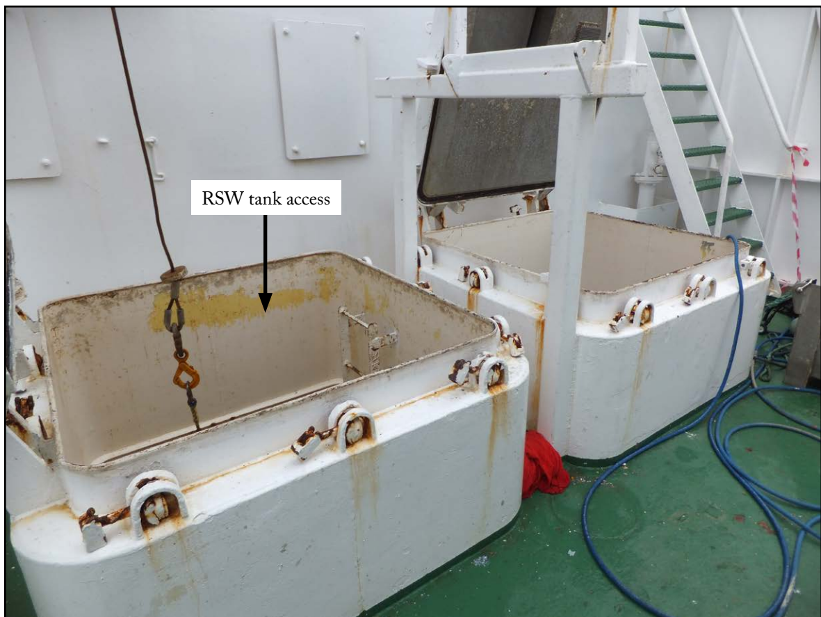
Figure 1: RSW tank access hatch
