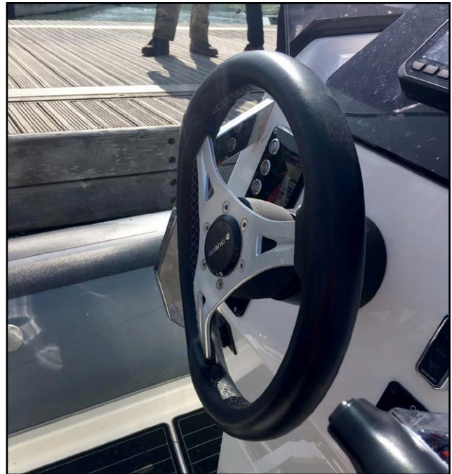
Figure 1: Buckled steering wheel
