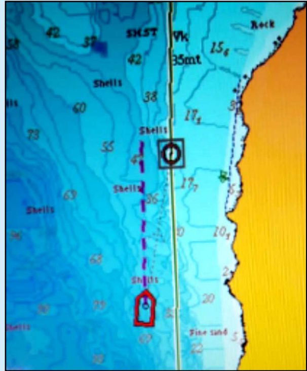
Figure 4: Zoomed out chart plotter view showing how the waypoint symbol (square) can obscure chart detail
