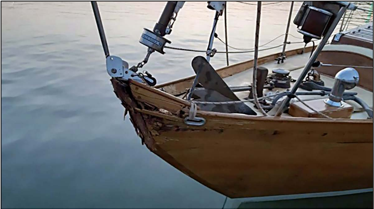
Figure 2: Damage to the classic yacht's bow
