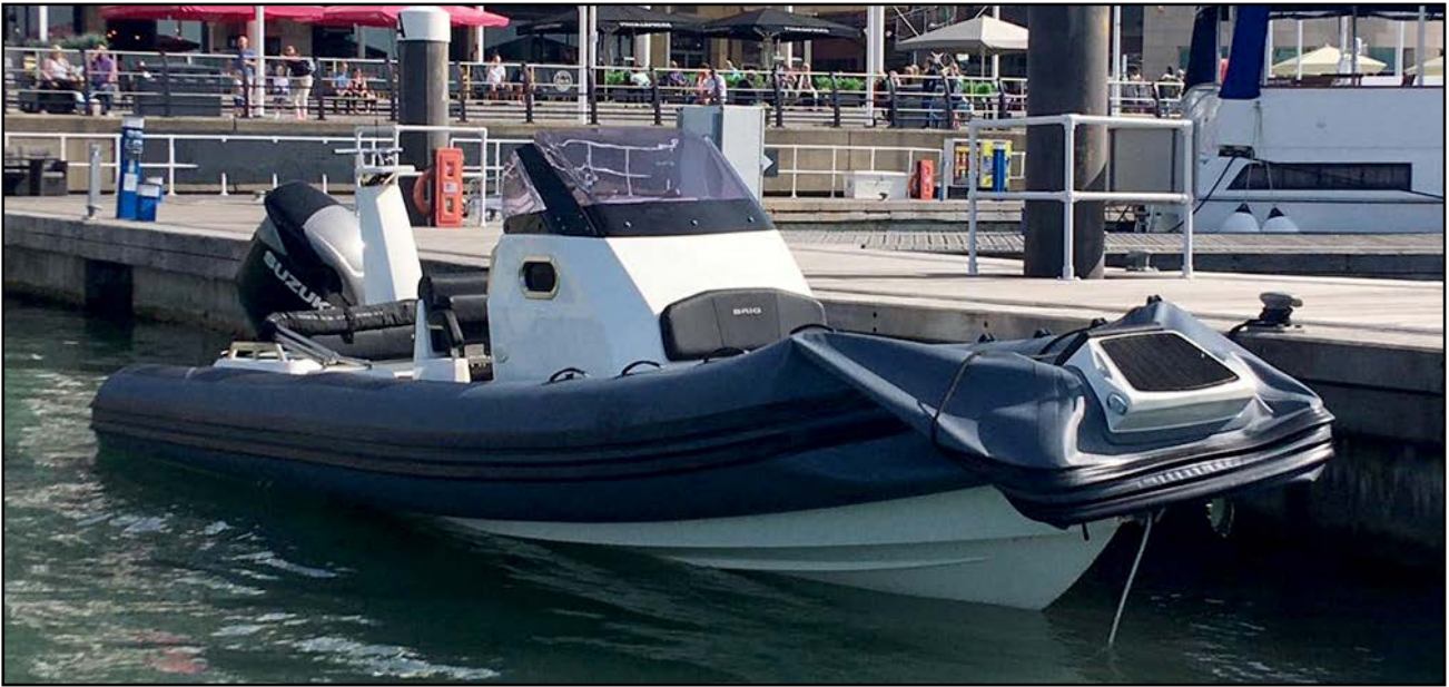
Figure 2: The RIB, showing damaged tubes
