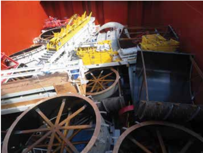
Figure 1.17 | An assortment of steel cargoes that has been improperly stowed and can cause delays in the vessel's discharge.
