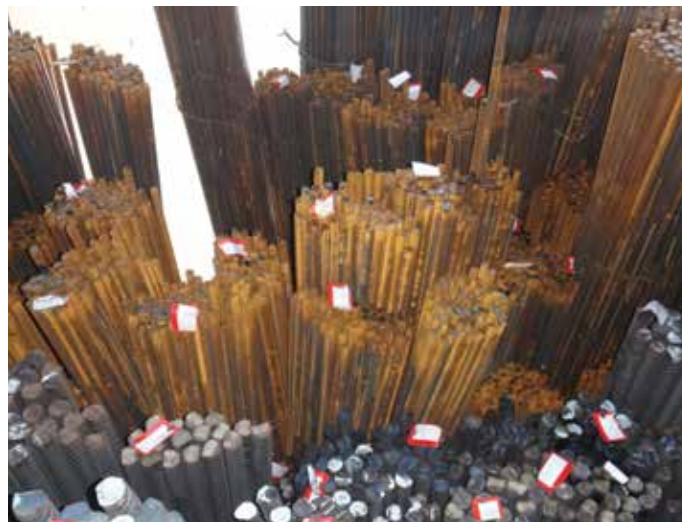
Figure 1.6 | Steel rebar stowed aboard the vessel at discharge port with bundles stowed on top and rusted due to water ingress through the hatchcovers while the vessel was in transit.
