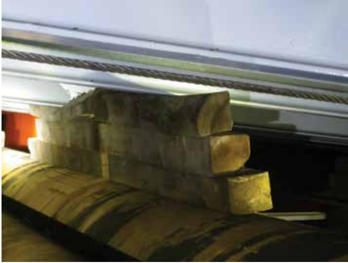
Figure 4.9 | Improper arrangement of dunnage that has been placed on top round shaped cargo.
