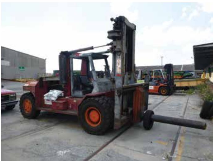
Figure 1.5 | Fork lift fitted with a tine specially designed for carriage of steel coil.
