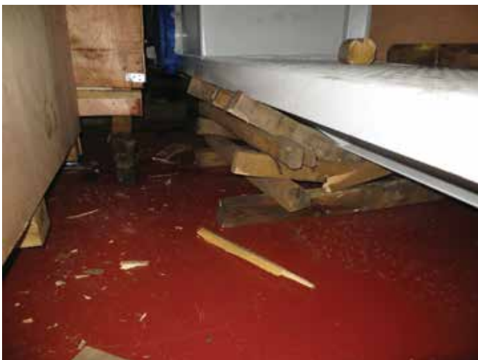
Figure 4.7 | Crushed dunnage caused the cargo stow failure.
