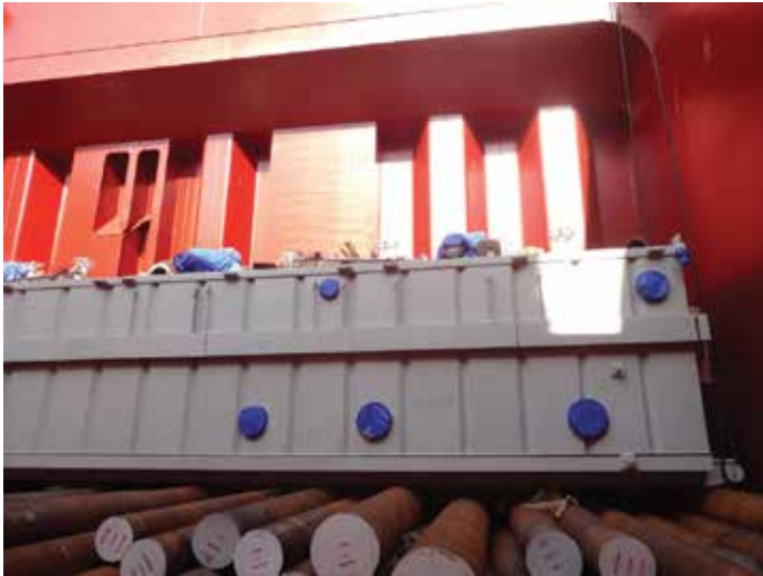
Figure 4.11 | Placement of cargo on the top of round shape cargo without proper dunnage.
