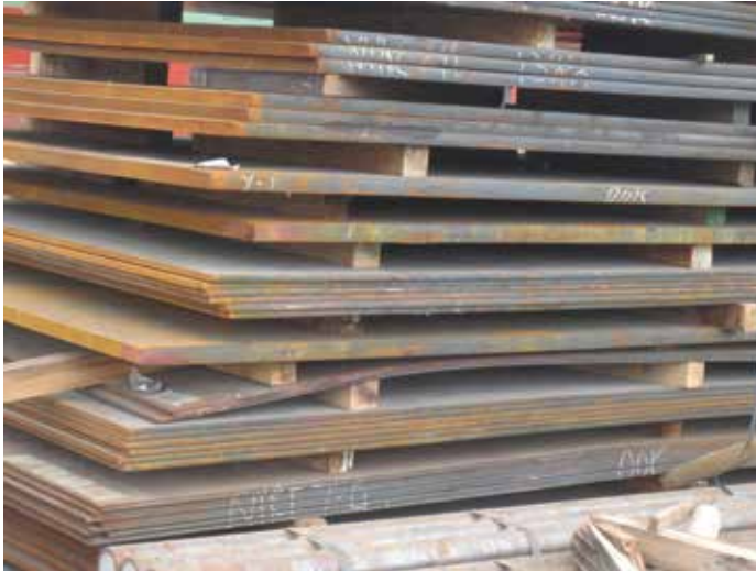
Figure 1.9 | Deformed steel plates due to non-vertically aligned dunnage.
