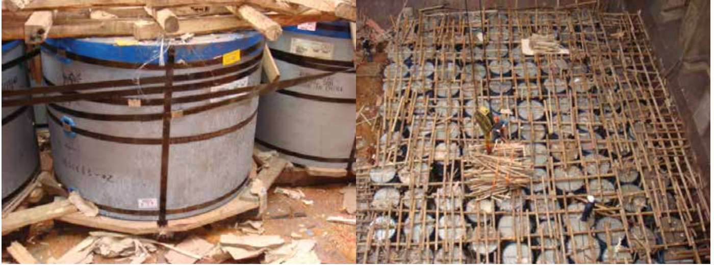
Figure 5.21 | Palletted steel coil stowed with “eye to the sky”.
