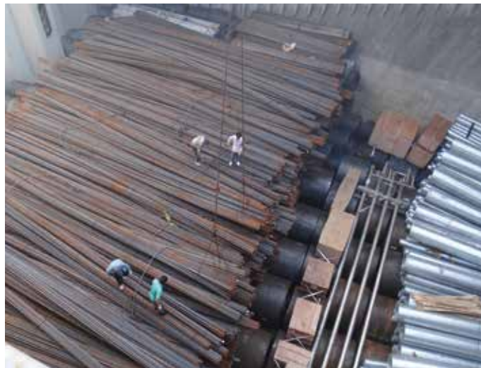
Figure 3.2 | Combination of steel cargoes being stowed, secured and lashed by stevedores.
