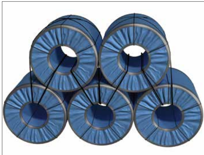
Figure 5.29 | Securing/lashing through centers of coils with 1 inch (2.5cm) wide flat steel band. Note that top-tier coils are banded in groups of threes to lower or adjacent coils depending upon the stowage configuration.
