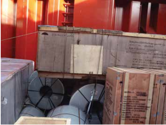
Figure 5.5 | Note that the wooden case is loaded on the top of steel coils.
