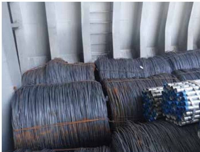
Figure 1.2 | Stowed steel wire and small diameter pipe. Note the deformation of the far left steel coil in the background as it is pressed against the side shell frame. This is particularly a concern for higher stacks of coils where lower tiers are pressed out towards the vessel's external bulkheads.
