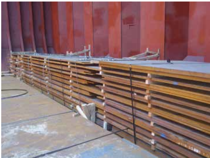
Figure 5.28 | Steel plates stacked athwartships against the bulkhead with proper dunnage and lashed/secured with steel band strapping.
