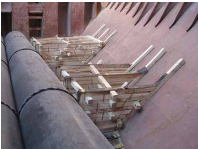
Figure 4.5 | Dunnage structures constructed on sloping hopper tank to hold large steel diameter pipes in place.
