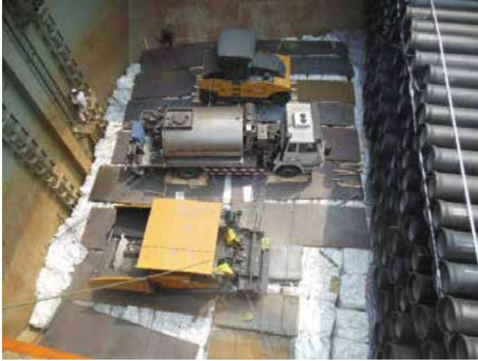
Figure 3.13 | Steel plates are placed on the top of bagged cargo to support vehicles and machinery adjacent to large diameter steel pipe that have been loaded in a fore and aft direction.
