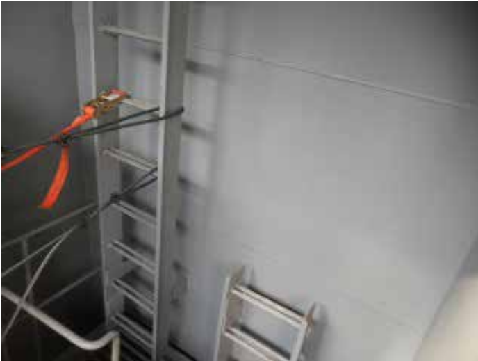
Figure 5.34 | Attaching lashings to the vessel’s structures, including ladders, as seen here should be avoided.
