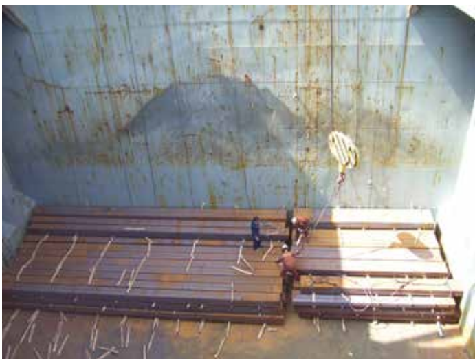
Figure 3.11 | Bundled steel channel are stowed in fore and aft direction inside cargo hold.
