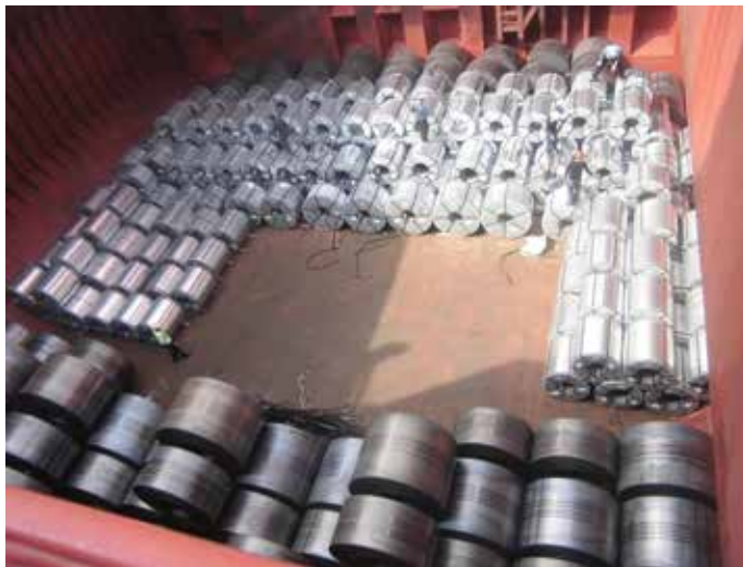
Figure 3.6 | Cold rolled steel coils being stowed and lashed with 1 inch (2.5 cm) wide flat steel bands in a cargo hold.
