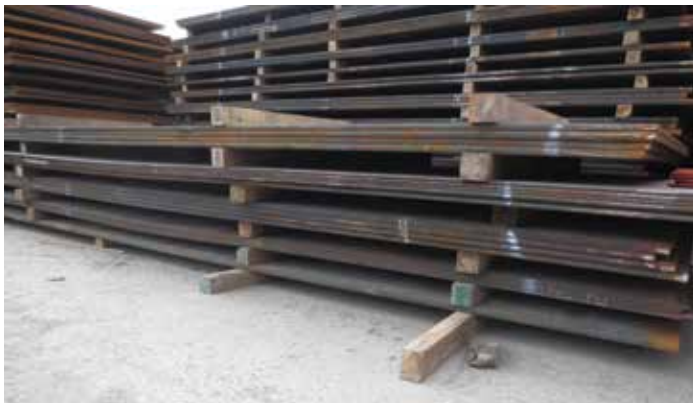
Figure 4.3 | Steel plates ashore awaiting shipment. Note the dunnage properly vertically aligned and horizontally spaced to prevent deformation of the stacked steel plates. The same stowage philosophy applies aboard the vessel for vertically stacked steel plates and steel plate bundles.
