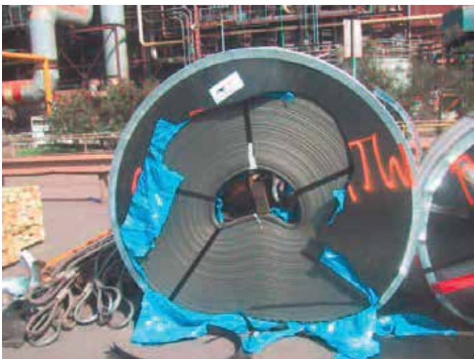
Figure 1.11 | Deformation to cold rolled coils due to excessive weight of loads on top.
