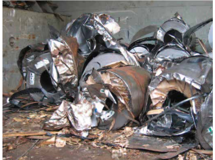
Figure 1.10 | Damage to coils due to cargo shifting.
