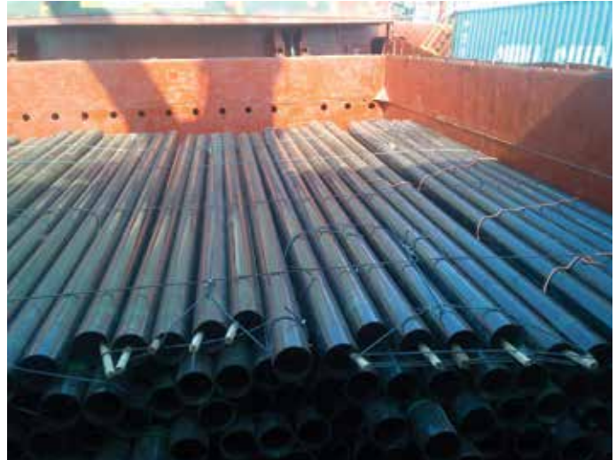
Figure 5.35 | Secured/lashed large diameter pipe. Note the dunnage wood inserted into the pipes in the foreground used for the lashing and securing of the top tier of stowed pipe.
