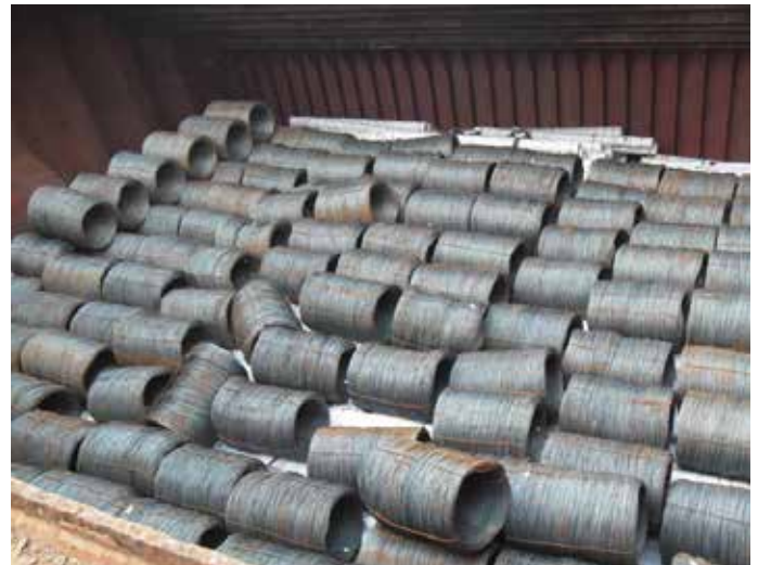
Figure 4.2 | Single and double tiers of coiled wire rod stacked on top packaged steel pipe.
