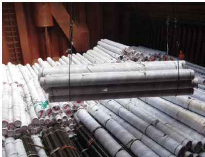
Figure 3.4 | Packaged and banded large diameter steel pipes being lowered into cargo hold.
