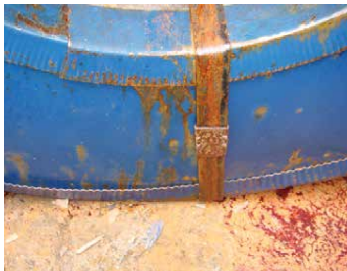
Figure 1.3 | Steel coil packaging damage resulting from cargo sweat during the voyage.
