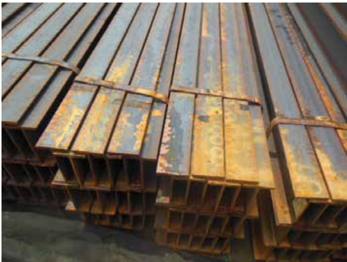
Figure 3.1 | Steel “I” bar stowed in an “in and out” position and secured with steel band.
