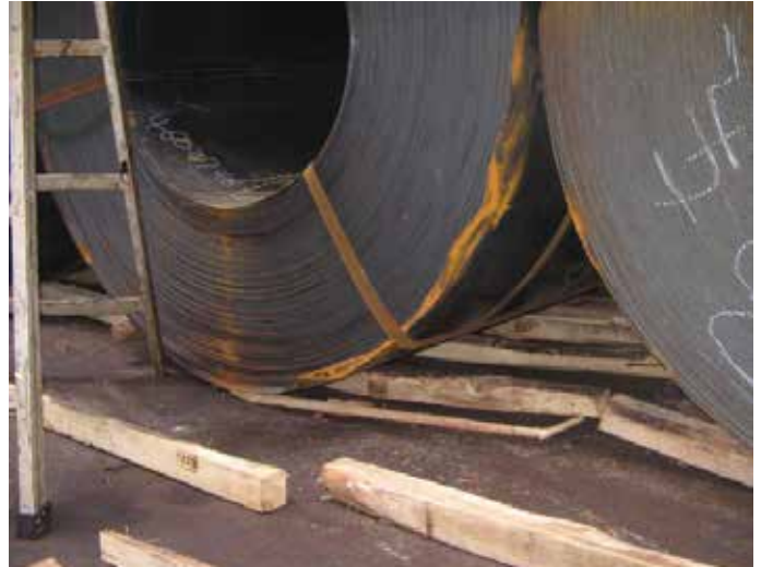
Figure 4.12 | Wooden dunnage that has been bent and crushed under the weight of steel coils.
