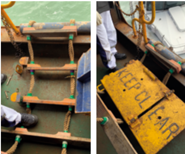
Pilot ladder incorrectly secured to the deck using D-shackles to choke the side ropes.
