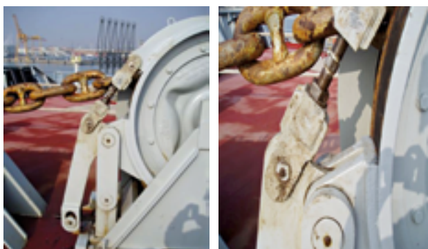
Brake 'Fully On' Bottle Screw Adjustment
