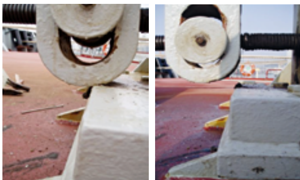
Incorrect Brake Adjustment Correct Brake Adjustment
