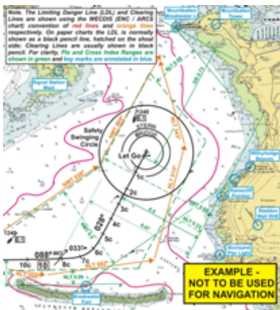
Figure 3 – Limiting Danger Lines and Clearing Lines. (Illustration courtesy of the Royal Navy).
