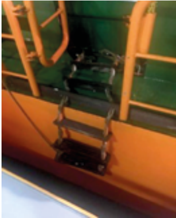
Another spreader used as a securing method.
