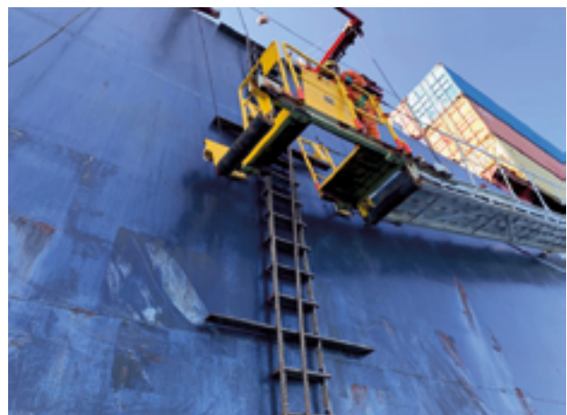
Compliant combination PBA with trap door – pilot ladder and man ropes extend up to and are made fast on vessel's deck
