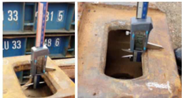
At ≈20mm the top plate thickness was 8mm thinner than more modern "flats" and the current industry standard, ≈28mm
