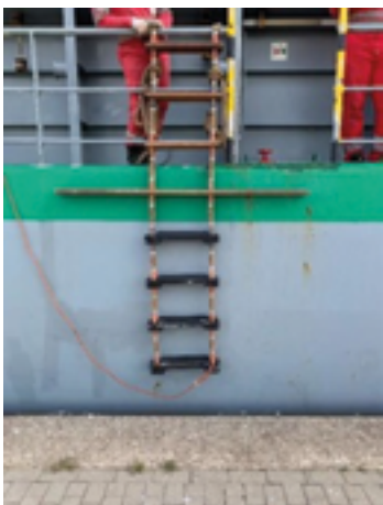
This setup means you have to stumble sideways to reach the entrance.
