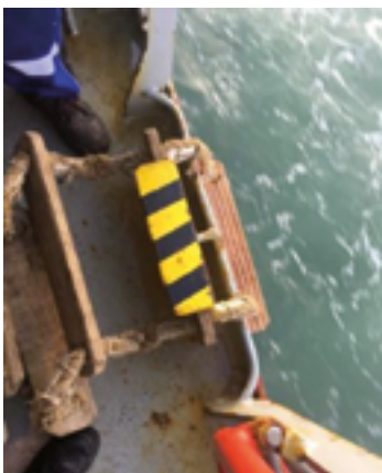
Deck tongue supporting the ladder.
