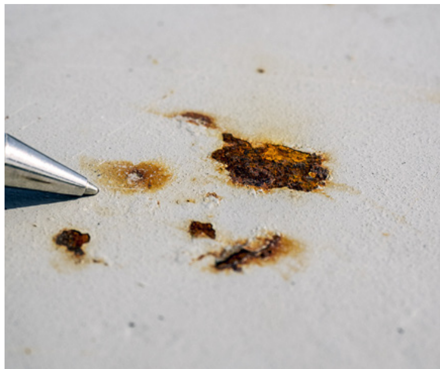
Fig 3. Premature breakdown of paint scheme on a coach roof resulting in vigorous corrosion of the exposed black steel. The total thickness of this scheme was just 60 µm (microns) which is a fraction of the 250 µm usually required.
