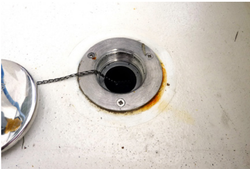
Fig 15. Rust developing around deck fittings owing to unprimed cut steel edges and lack of adequate bedding compound.
