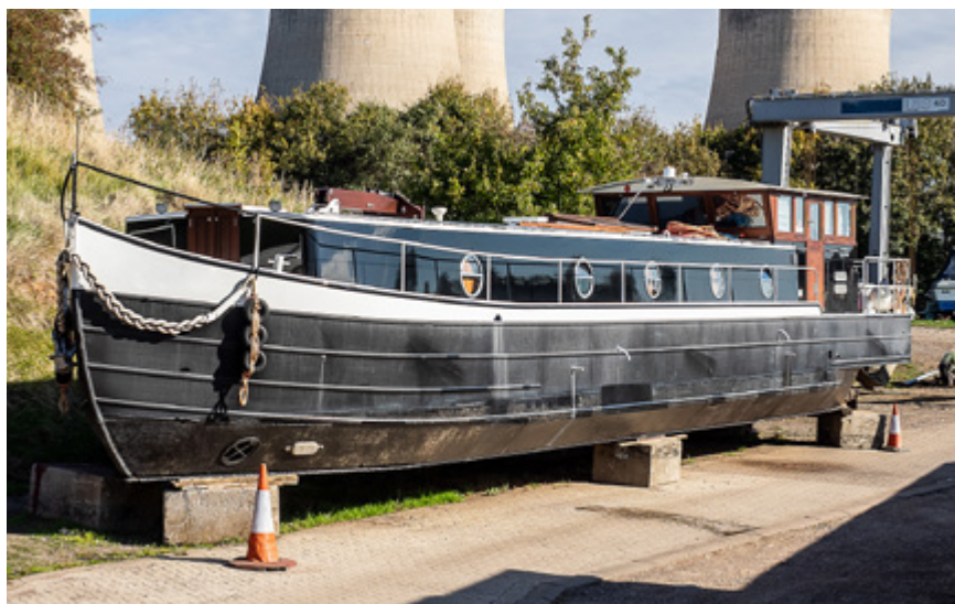
Fig 9. A similar Dutch Barge on hardstanding. Note the length of the solid bulwarks and the lack of adequate water freeing ports.
