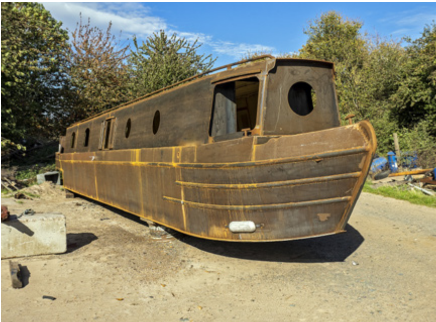
Fig 1. This newly fabricated narrowboat is being allowed to rust in the open to help remove millscale. The loosened millscale can be removed by wire brushing before primer is applied. Preparation is not as good as blast cleaning but is preferable to painting over millscale.
