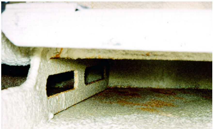
Fig 12. Unprimed steelwork corroding in void space beneath an aft deck. Spray foam provides little anticorrosive protection whilst chemicals used in spray foams will encourage rather than inhibit corrosion, especially if applied to aluminium.
