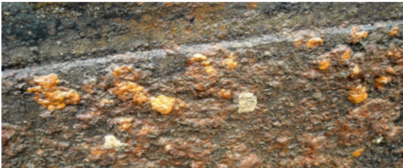
Photograph 2 - Extensive Gallionella Ferruginea attack on a Narrowboat
