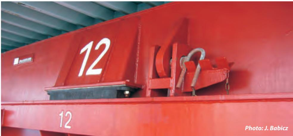
**Flexipad** – A non-sliding flexible bearing pad developed by MacGREGOR. It is made up of flat layers of steel and rubber, bonded together and mounted on a steel plate. The load on Flexipad from the weight of the hatch cover and cargo causes some compression in its rubber elements. A horizontal load causes a sideways deflection of the rubber layers. In general there is no sliding of the pads on the coaming to cause bearing surface wear.
