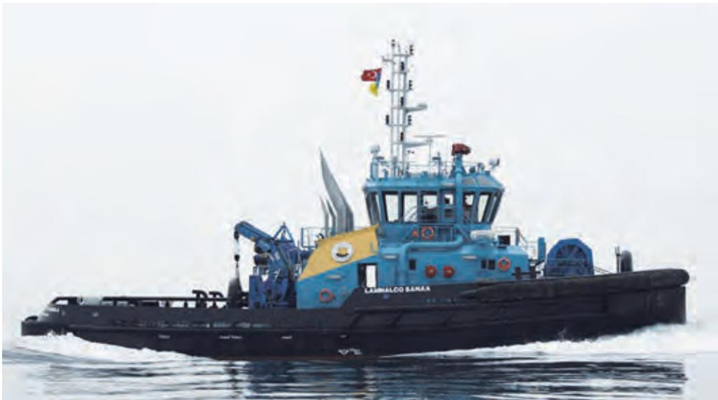
The principal particulars of this RAstar 3600 Class tug are: Length, OA: 35.80m, Beam, moulded: 14.50m, Depth, moulded: 6.03m (above design baseline), Maximum operating draft: 6.50m (to underside of drives), Bollard pull, ahead/astern: 118t/110t maximum, Free running speed, ahead: 15.1 knots, Lightship mass: 963t.
