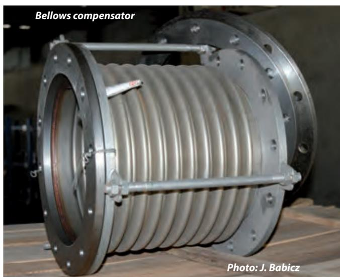
**Bellows** – A thin metal cylinder with corrugated walls to permit reasonable deflection under applied pressure.
