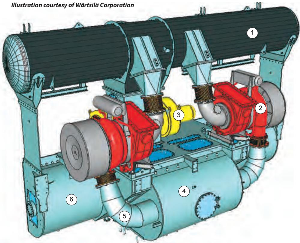
**Complete scavenging system for Wärtsilä SULZER RT-flex60C engine, comprising exhaust manifold "1", two turbochargers "2", auxiliary blowers "3", scavenge air cooler "4", scavenge air pipes "5", and scavenge air receiver "6"**
