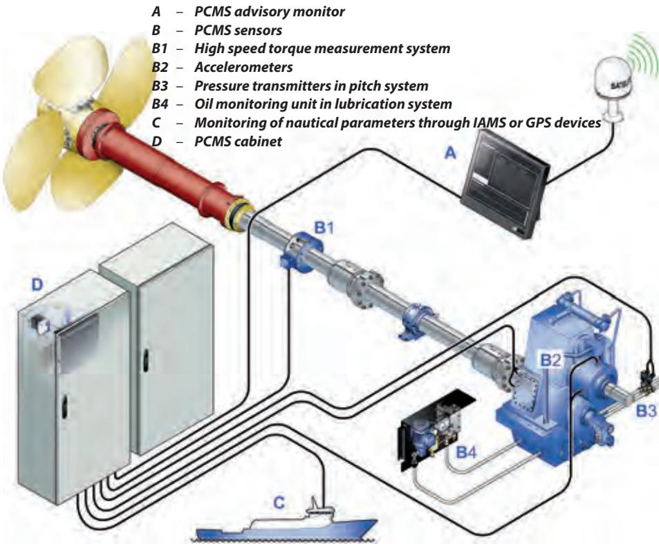
The number of inputs can be changed depending on the specific requirements. Accelerometers are used to monitor the condition of mechanical parts, such as gears and bearings, but can also detect for example, blade damage. One PCMS system can process up to 16 accelerometers simultaneously. Lubrication and hydraulic oil is monitored by measuring temperature, the oil-water saturation, and any oil contamination.
