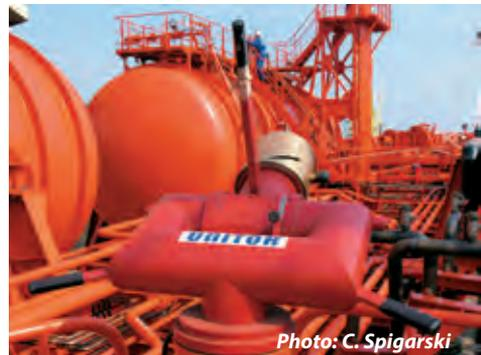
**Fire monitor** – Fixed foam/powder/water cannon shooting fire-extinguishing agents on the tank deck, manifold etc.
