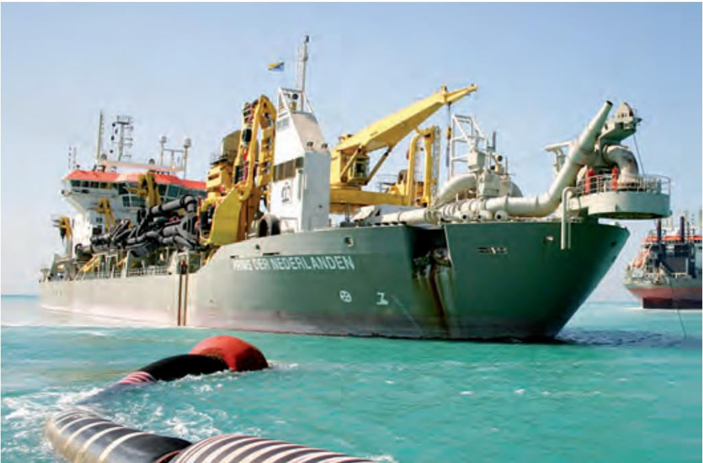
*Discharge can be made directly into a floating shore delivery pipeline using a ball joint connection over the bow and a discharge pump. A rainbowing nozzle is provided to spray the mixture directly over the bow.*
