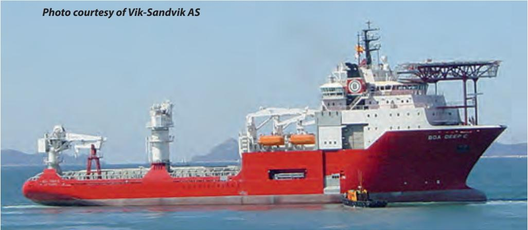
guide winches and powered guide pins also installed. BOA DEEP C also boasts twin built-in deepwater ROVs of Oceaneering Millenium type and a 7.2m x 7.2m moonpool. The ROVs are located in hangars. Over the side a guided launching system for extreme condition operation is provided.
