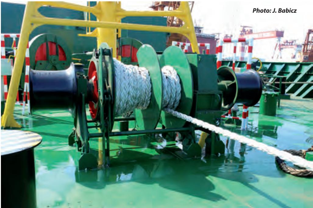
**Three speed pole-change drive** – The nearly maintenance-free electric motor is equipped with standstill heating, temperature sensors and fail-safe brake. The winch control is precise and easy. Speed steps in both directions are obtained by a single lever. Electric systems are easy to install and provide quick start in all environmental conditions.
