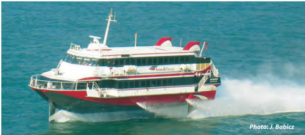
**Hydrofoil, hydrofoil boat** – A vessel with underwater wings (hydrofoils) fitted below the hull. The dynamic lift of hydrofoils keeps the hull clear of the water surface while underway. The hydrofoils provide a substantial reduction in resistance with ability to maintain speed in rough seas. The foils, attached by struts to the hull, may either pierce the water surface, or be totally submerged.
