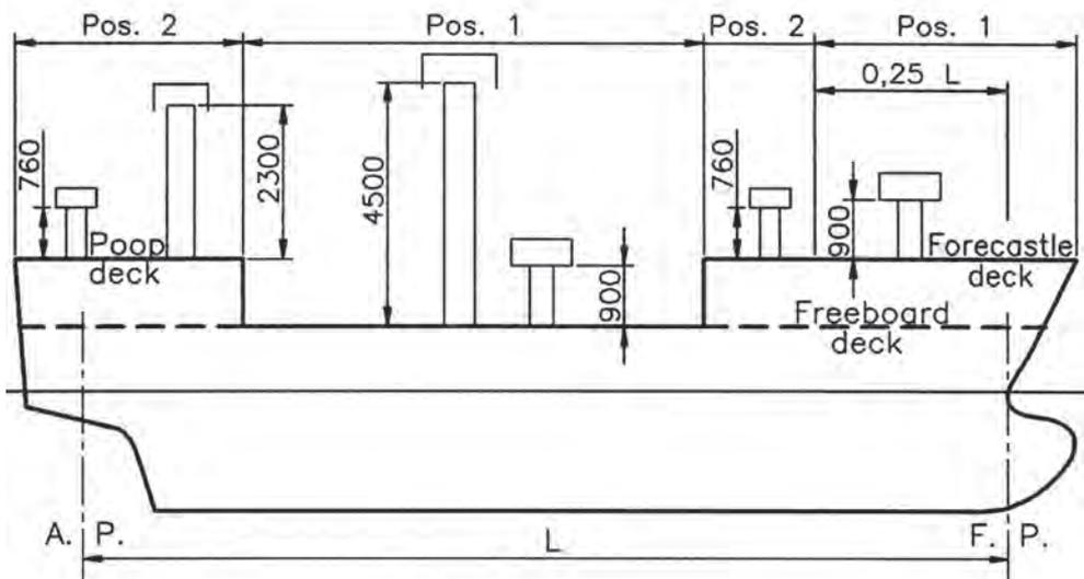
**International Convention on Load Lines; Required ventilator coaming heights (mm)**
