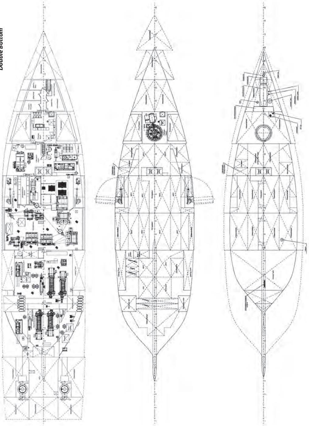
Length (oa): 94.8m, Breadth: 19.2m, Draught (max): 6.5m, Speed: 15 kn, Class: GL + 100 A5 E3 Nav-OC (special vessel) + MC E3 AUT RP3 50% strengthened to Polar Class PC 7
