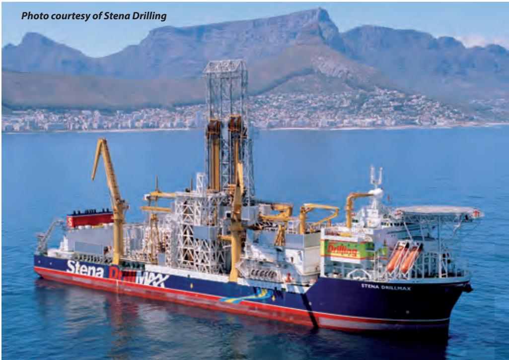
*The world's largest drilling ship STENA DRILLMAX, built by Samsung Heavy Industries in Korea has twin drilling derricks and is intended for oil and gas exploration in water up to 3000m. With a displacement of 97,000t, overall length of 228m and breadth of 42m, it is capable of drilling to a depth of 11,000m.*
