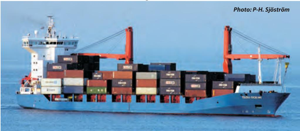
*Feeder vessel: note the enclosed bridge*
