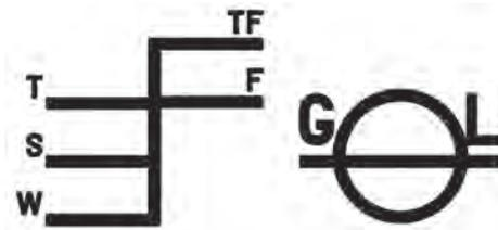
(provided in tabular form) and correcting it for those geometric properties of the ship which differ from those of the standard one. There are corrections for block coefficient, depth, superstructure, trunks and sheer. The result of this calculation, the load line mark, is permanently marked on the ship hull.
