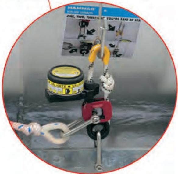
**Hydrostatic release unit (HRU)**
