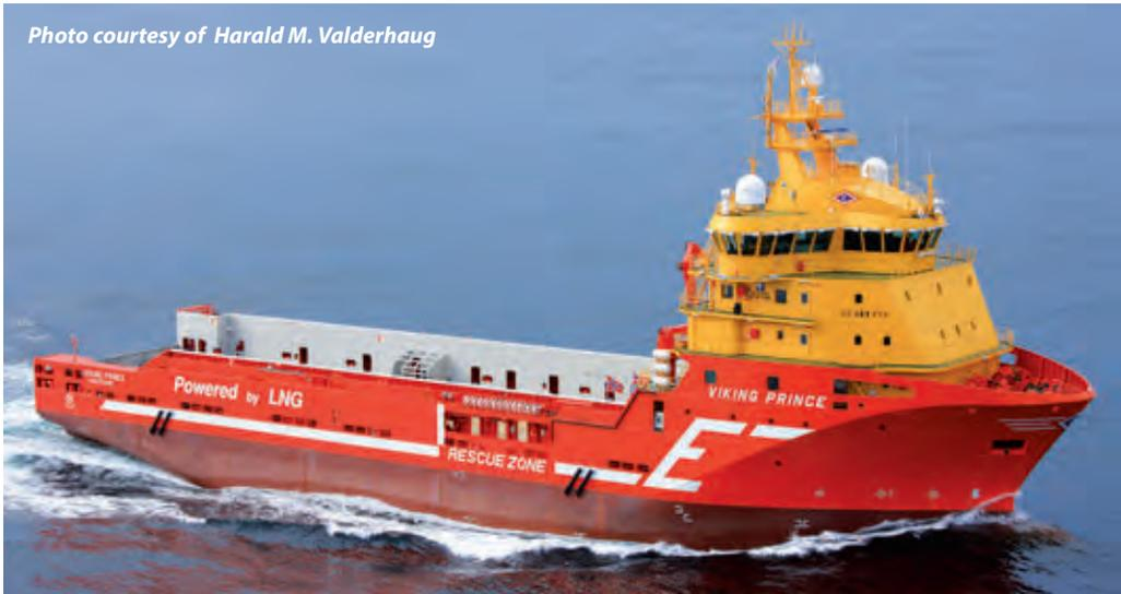
*The general layout of PSVs has become fairly standardized, with a large open working deck aft and the accommodation forward. They have low angle of deck immersion due to small depth in way of open working deck*
