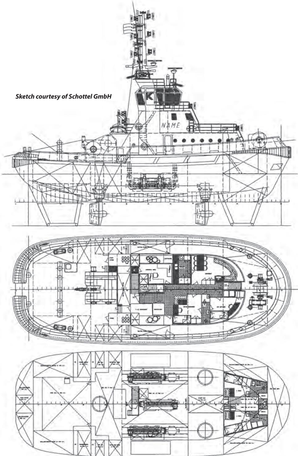
unit, incorporating a five-blade fixed pitch propeller of 2.15m diameter and a **Kort nozzle**. Power is transmitted through Twin Disc type 3000-2LD Marine Control Drive (MCD) units. The main engines are sited "side by side" across the engine room, with the outboard engines coupled to the forward Schottel units and the center engine driving the aft unit. On trials the tugs produced a bollard pull ahead of 75 tonnes and 73.5 tonnes astern, with a free-running speed of 12 knots.
