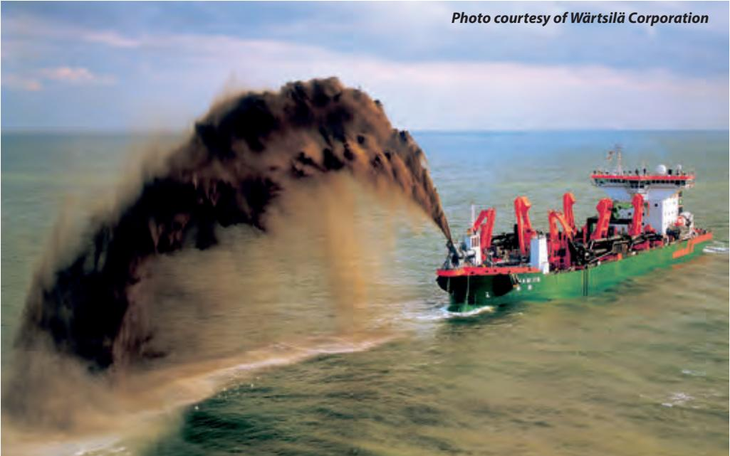
The mixture can also be jetted forward over the ship bow via a mixture jetting nozzle (rainbowing).
