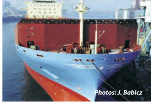
*Standard breakwater on the 2200TEU container vessel*
