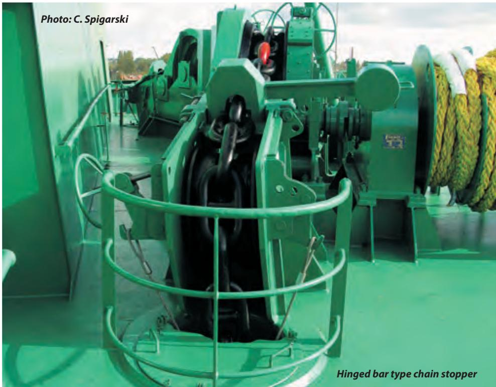
the housed position in the **hawse pipe**. **Chain stopper** usually consists of two parallel vertical plates mounted on a base with a pivoting bar or pawl which drops down to bear on a chain link.
