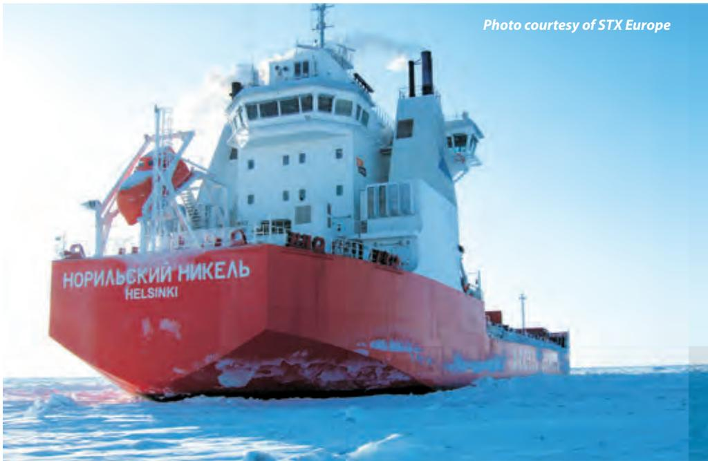
**Double-acting container vessel NORILSKIY NICKEL**
