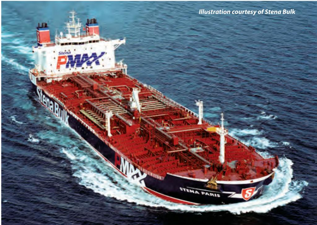
Length, oa: 182.90m, Length, bp: 175.50m, Breadth, mld: 40.00m, Depth, mld to main deck: 17.90m, Draught, design/scantling: 11.30/13.00m, Deadweight, design/scantling: 54,0001/65,200dwt, Cargo capacity: 70,200m<sup>3</sup>, Main engine output: 2x7860kW at 129rev/min, Service speed: 14.50knots, Complement: 26.
