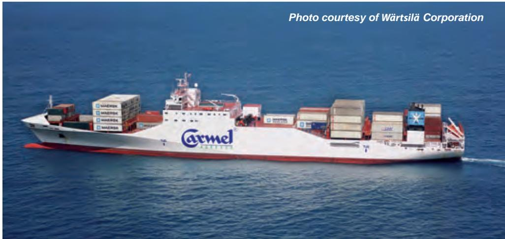
An interesting feature is the adoption of an innovative arrangement with the **superstructure** located amidships above the large, fully-insulated refrigerated hold. Three conventional cellular holds are placed forward of this hold and two aft, offering places for 266TEU. Additional 630TEU can be carried on hatch covers and open deck provided with **lashing bridges**.
