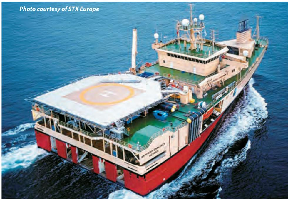
The maximum beam, equivalent to half of its length, is at the transom, giving the vessel its shape. The broad transom allows for efficient seismic equipment handling and provides for a large working area both on the aft deck and in the instrument room. The Ramform-type hull has good motion characteristics, even in rough weather, accelerations at the stern of the ship are modest.
