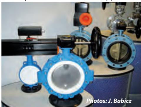
**Butterfly valve** – A rotary stem valve with a centrally-hinged disc of the same diameter as the pipeline. The valve opens into the pipeline and therefore takes up little space, permits large flow rates and gives minimum pressure drop.
