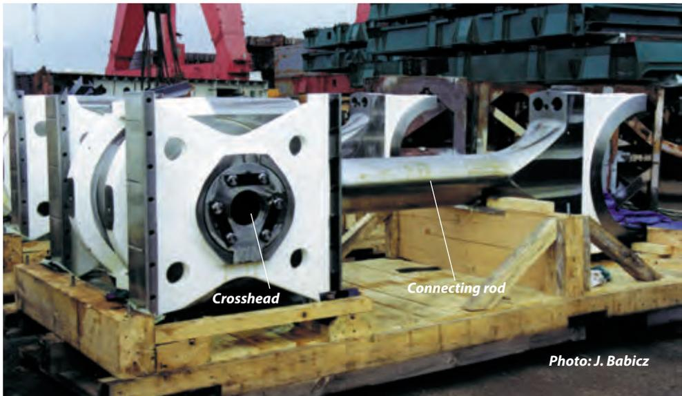
**Crosshead** – A reciprocating block which usually slides in guides and is the connecting point for **piston rod** and the **connecting rod** in a low-speed, two-stroke diesel engine or for rams and tiller in a **steering gear**.
