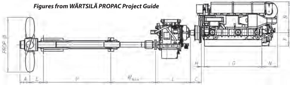
**Propac CP – propulsion system**
