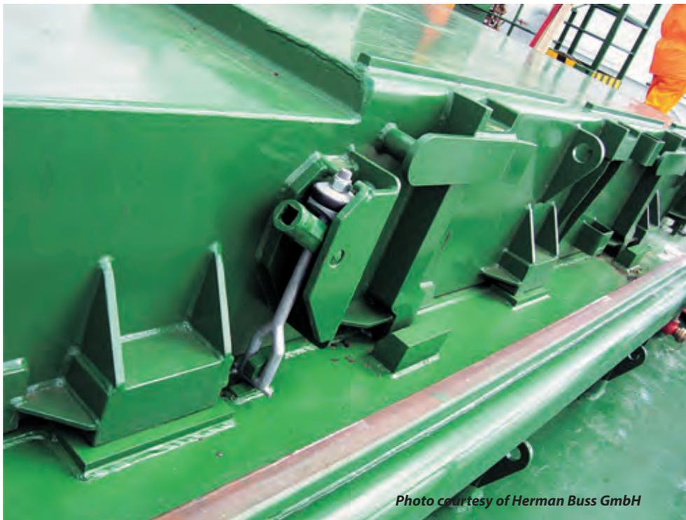
**Quick-acting cleat**, battening device – A cleat applied manually by a lever to provide the necessary locking. **Hatch covers** are secured to the coaming by quick-acting cleats. The cleat consists of an eyebolt and a cam. The length of the cleat is adjusted by a nut. The necessary resilience is produced by a rubber washer being compressed in between steel washers.
