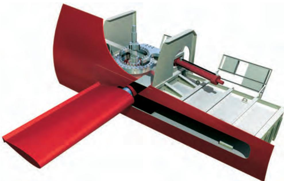
*The Brown Brothers Aquarius folding stabilisers designed for small cruise ships, passenger ferries, small naval and coastguard vessels. Fin area: 1.82 - 5.78 m<sup>2</sup>, total weight: 19.3 - 40.2 tonnes.*
