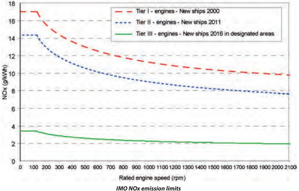
The IMO Tier 2 NO<sub>x</sub> emission standard entered into force on 1st January 2011 and applies globally for new marine diesel engines over 130 kW installed on ships which keel laying date is 1st January 2011 or later. IMO Tier 2 NO<sub>x</sub> emission levels correspond to about 20% reduction from the IMO Tier 1 NO<sub>x</sub> emission standard. This reduction is reached with engine optimization.
