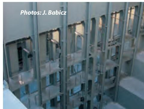
**Container cell guides** – Containers are commonly stowed below deck and sometimes on deck within fixed vertical cell guides, which guide them into place and ensure that they do not move during the voyage.
