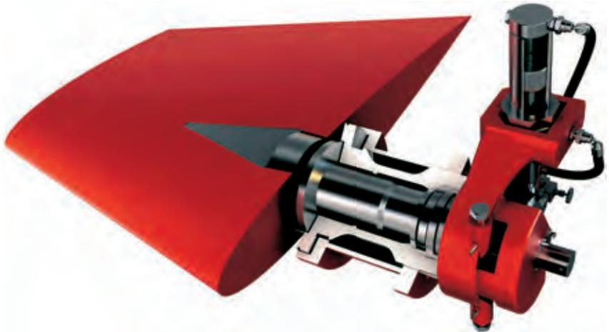
***The Brown Brothers Gemini non-retractable stabilisers designed for smaller vessels.
