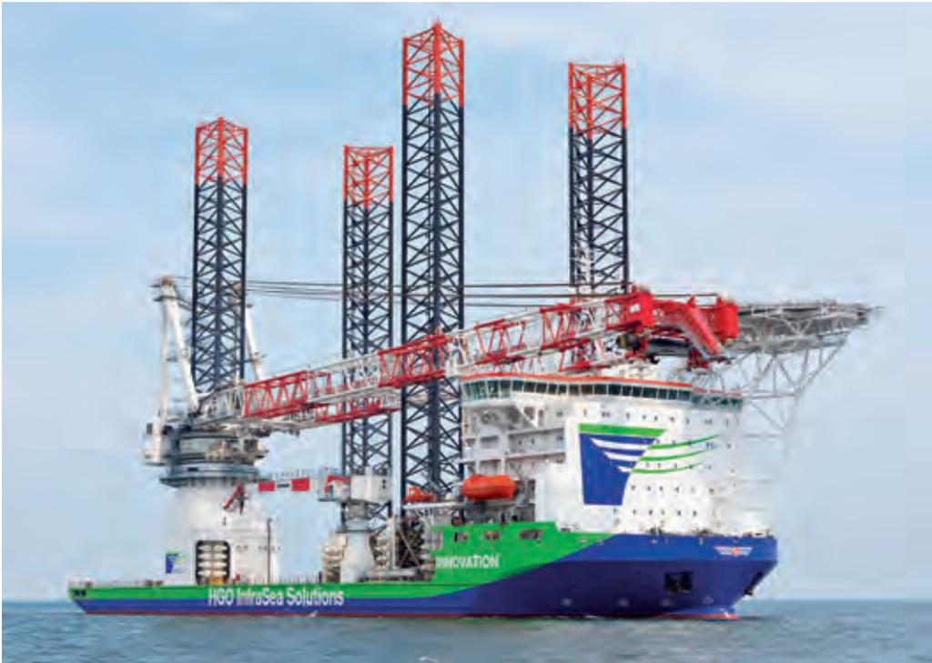
The vessel is equipped with 4 independent legs of 3-Chord truss type with spud cans and high speed Rack and Pinion Jacking System. The system consists of 96 elevating units, divided into 4 layers and is able to operate even if one layer is lost.
