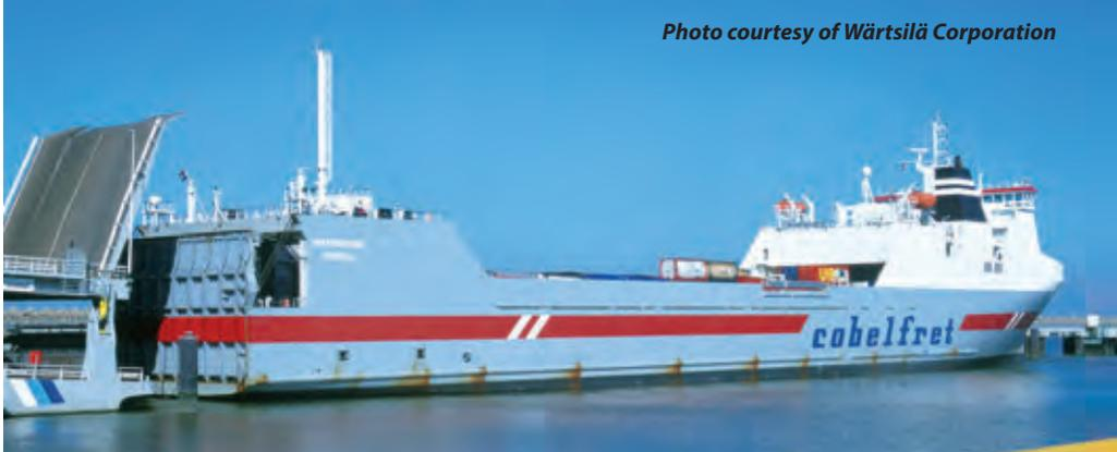
*The ro-ro paper product carrier SPAARNEBORG and her two sisters are each powered by a Wärtsilä Sulzer 7RTA52U main engine of 10,920kW, and two Wärtsilä 6L20 auxiliary engines, each of 980kW. All engines are equipped with SCR systems to reduce NOx emissions to the minimum*
