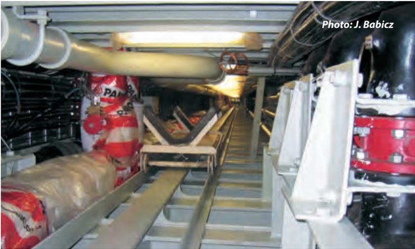
**Pipe tunnel** – The void space running in the midships fore and aft lines between the inner bottom and shell plating forming a space for ballast, bilge and/or fuel lines.
