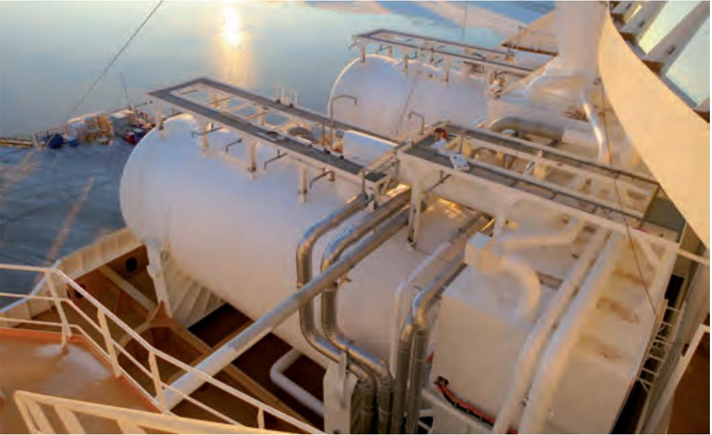
Wärtsilä's patented Cold Recovery System utilises the latent heat of LNG in air conditioning systems, reducing the amount of electricity consumed in cooling compressors. Significant operational savings and an increase in overall vessel efficiency are the result.
