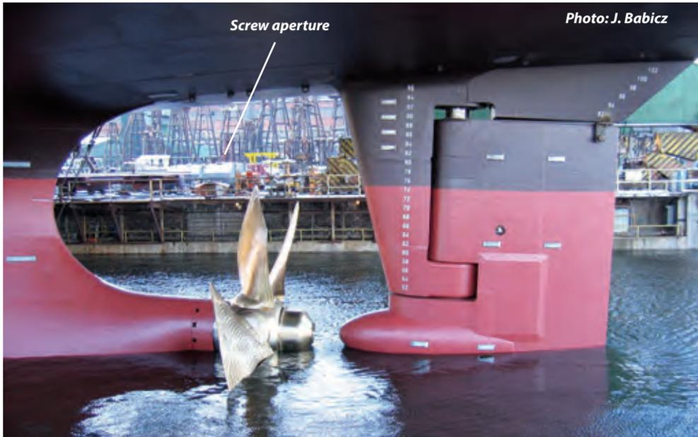
**Screw aperture** – The opening aft of the **stern frame** in which the **propeller** rotates. See also **Propeller clearances**.
