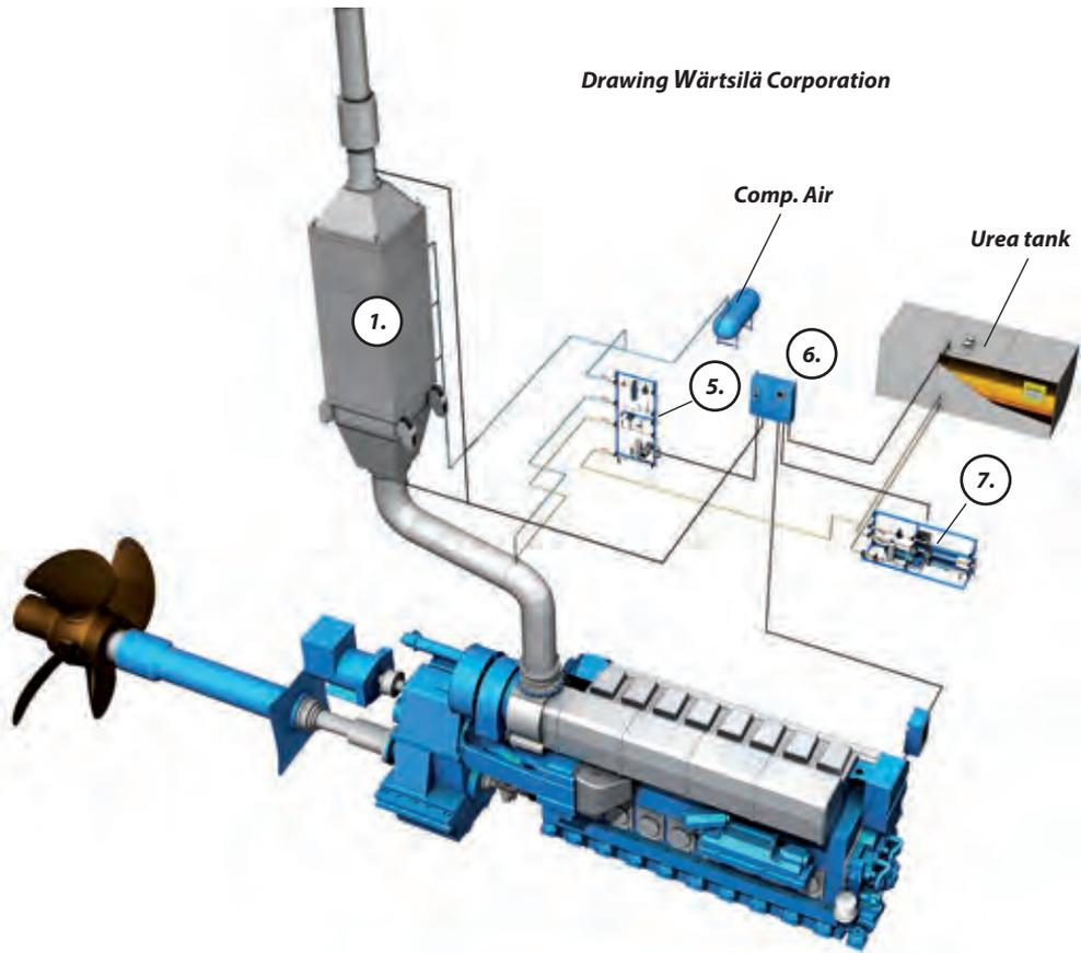
The dosing unit defines the correct urea dosing rate for the injection system and adjusts the urea flow accordingly by a control valve. The components in the unit are mounted on a frame, forming a compact module. One pump unit can be used for several SCR reactors while one dosing unit is installed for each SCR reactor.
