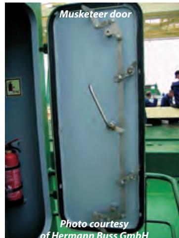
**Musketeer door** – Marine door with a novel locking mechanism developed by WINEL Company (the Netherlands). The Musketeer locking system incorporates a 33:1 power transmission from manual operating force to the locking device; as a result the door can be securely locked and opened even using an elbow or a shoulder only.
