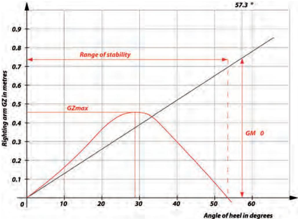
**Curve of righting arm GZ, curve of static stability** – The plot of the righting arm GZ calculated as function of the heel angle at constant **displacement** and vertical centre of gravity KG.
