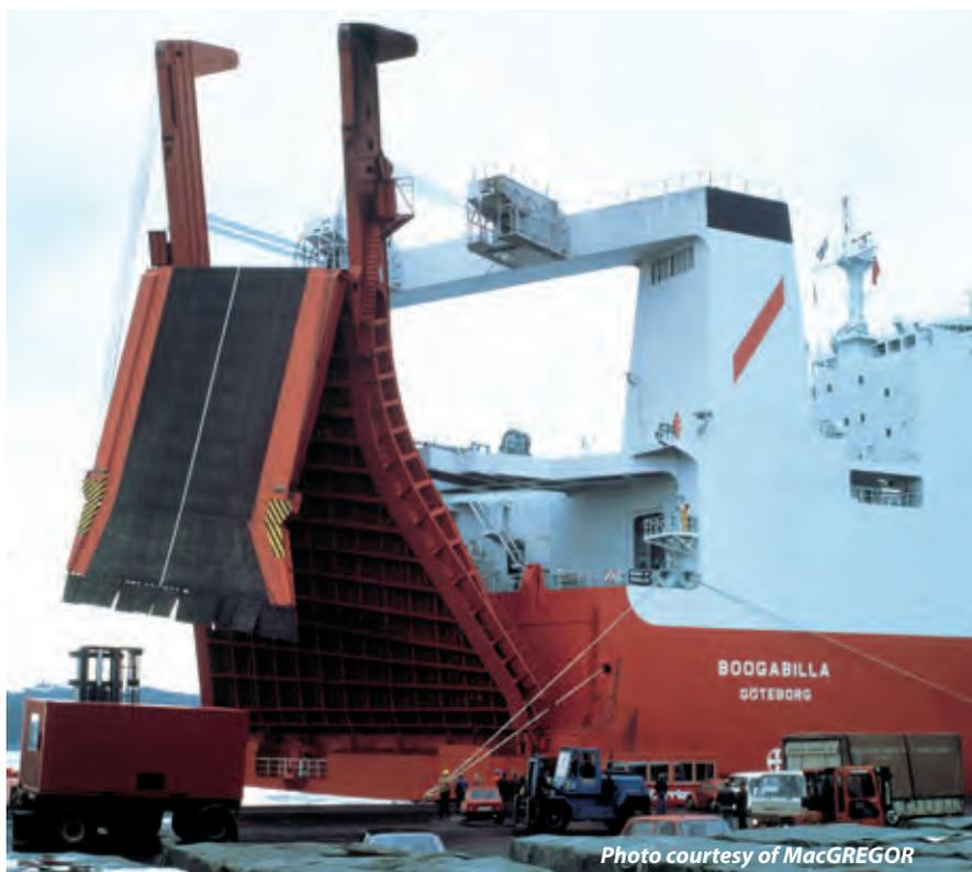
Ro-ro vessels berthing at quays with considerable height differences require long ramps. To avoid storage problem, foldable stern ramps can be used. The foldable stern ramp/door comprises two main sections articulated together and provided with outer and inner flaps to allow smooth transition of vehicles. When in the closed position, the inner section acts as a weathertight door, secured by hydraulically-operated cleats and locking devices.
