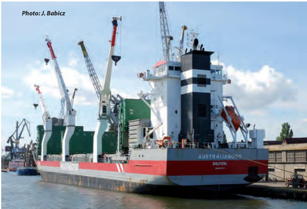
**Multi-purpose cargo ship** – The vessel designed for transport of wide range of commodities such as general cargo, forest products, dry bulk, grain, steel coils and usually equipped for transport of containers. Such vessels have tank top strengthened for heavy cargo and grab operation. Permissible tank top loading 10-20t/sqm.
