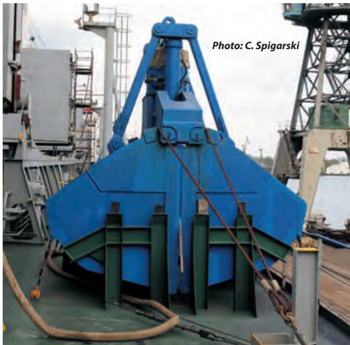
**Grab** – A bulk cargo-handling device consisting of a bucket which is hinged to open and close. It is open when lowered into the cargo and then closed and lifted out full. It is opened to discharge the cargo ashore, or into the ship cargo hold.
