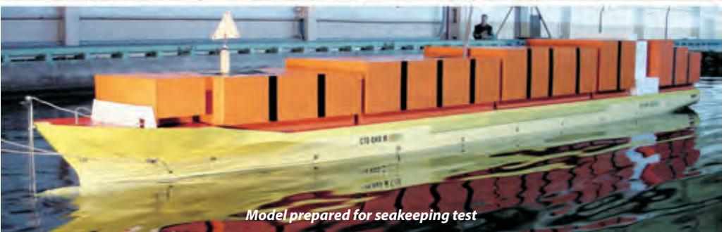
*Model prepared for seakeeping test*
