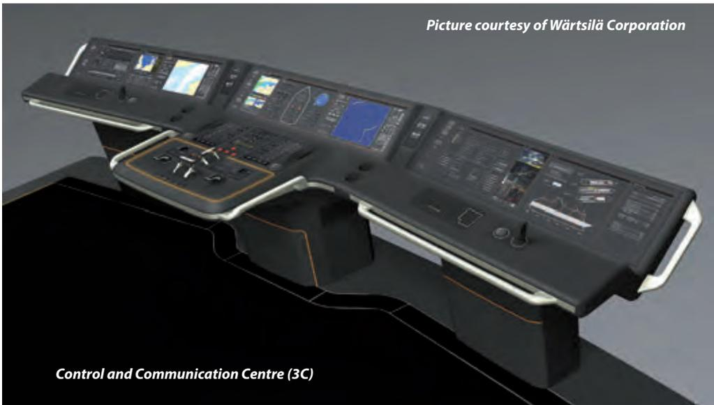
**Control stations** – Those spaces in which the ship radio or the main navigating equipment or the emergency source of power is located, or where the fire recording or fire control equipment is centralized, (SOLAS).
