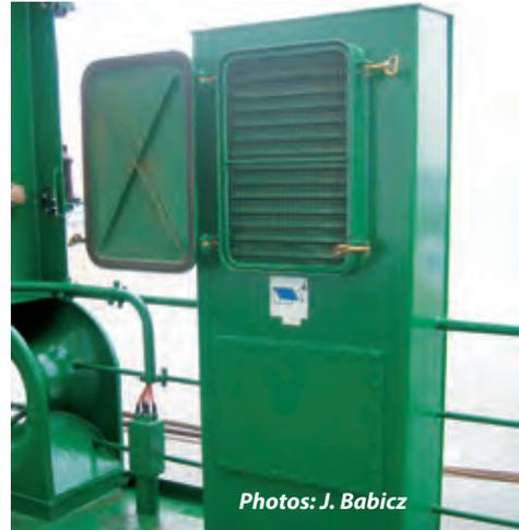
**Ventilator** – Any grid, vent pipe or opening through which air can enter or leave a space. Vent pipes on the weatherdeck can be a source of water ingress to lower deck areas. Strong built-in vent trunks are safer solutions.
