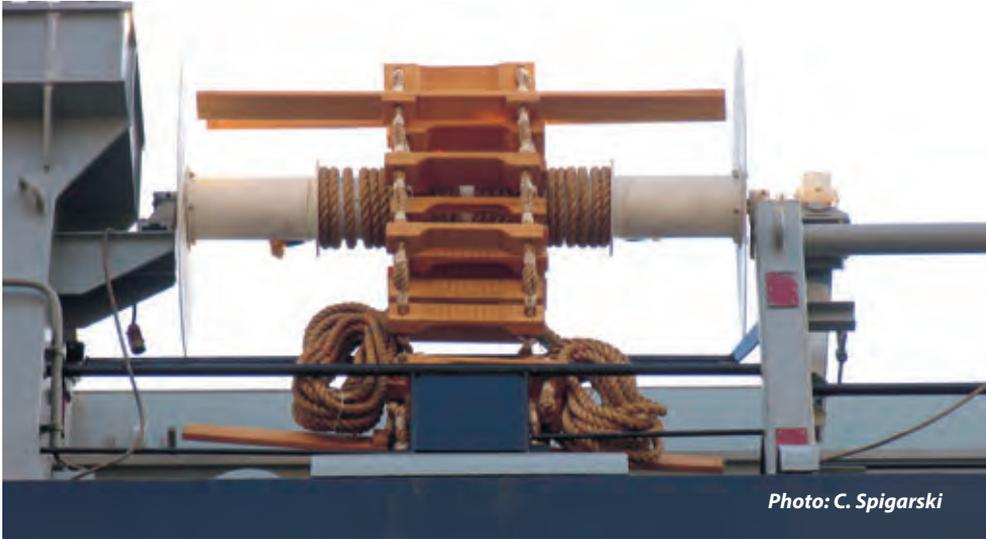
**Note:** Pilot ladders on stowage drum tend to stay clean, are easy to rig, retrieve and survey, and they last longer too. However, the drum should NOT be used to hoist/lower a pilot from/to the pilot boat.
