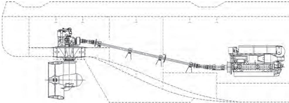
**Propac ST – arrangement with fixed propeller thrusters, cardan shafts and slipping clutch**
