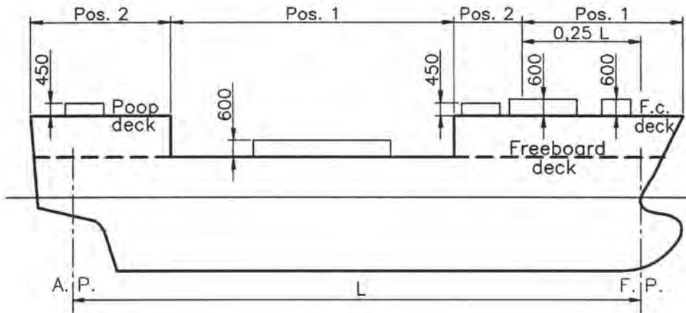
**International Convention on Load Lines; Required coaming heights (mm) of hatches**
