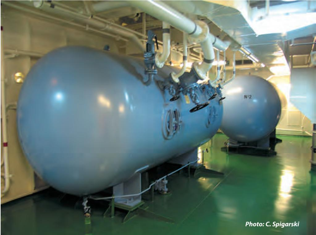
*Air receivers onboard the 4444 TEU container vessel
