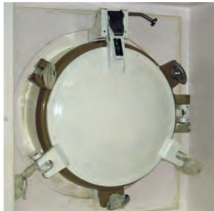
Sidescuttles are divided into three types: Type A (Heavy), type B (Medium) and type C (Light). The minimum requirement for type A is that it shall withstand a water pressure
