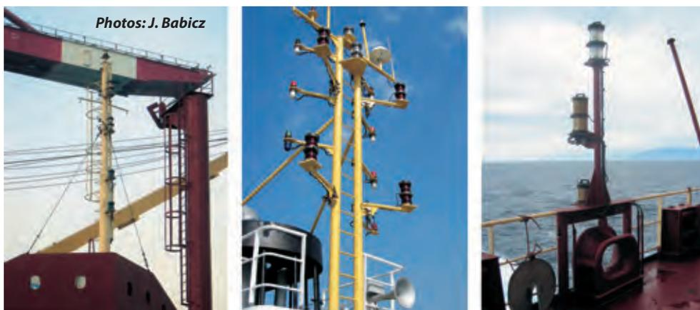
**Navigation lights** – All seagoing ships must be equipped with running and signal lights in compliance with the International Regulations for Preventing Collision at Sea (COLREG). A navigational light panel is installed in the **wheelhouse** for the control of all running and signal lights.
