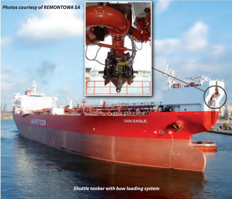
Shuttle tanker with bow loading system
