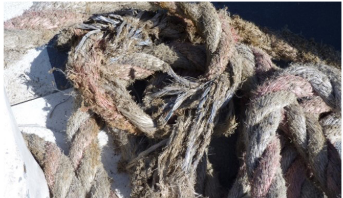
Figure 8B | Fleet ropes in poor condition
