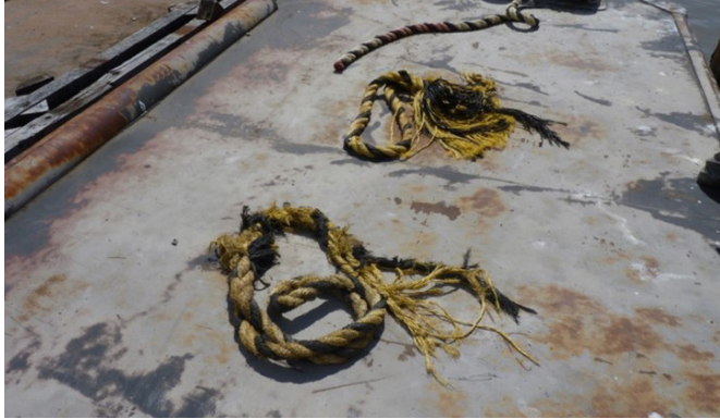
Figure 8C | Fleet ropes that parted
