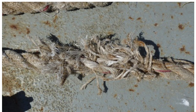
Figure 6B | Lines in poor condition
