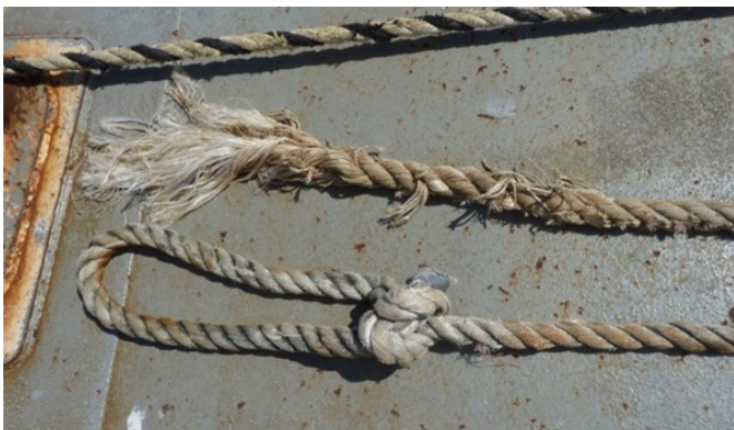
Figure 6A | Lines in poor condition
