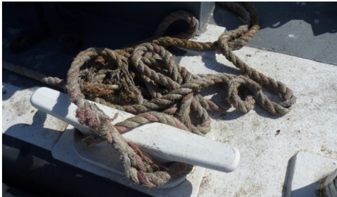
Figure 8A | Fleet ropes in poor condition
