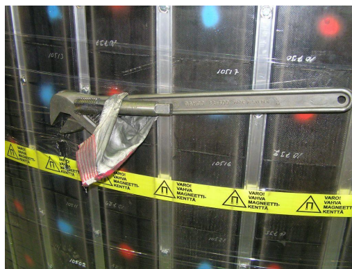
Ferromagnetic tools cause real danger
