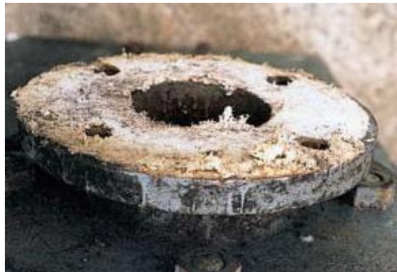
Remains of Asbestos (of flange gasket)
