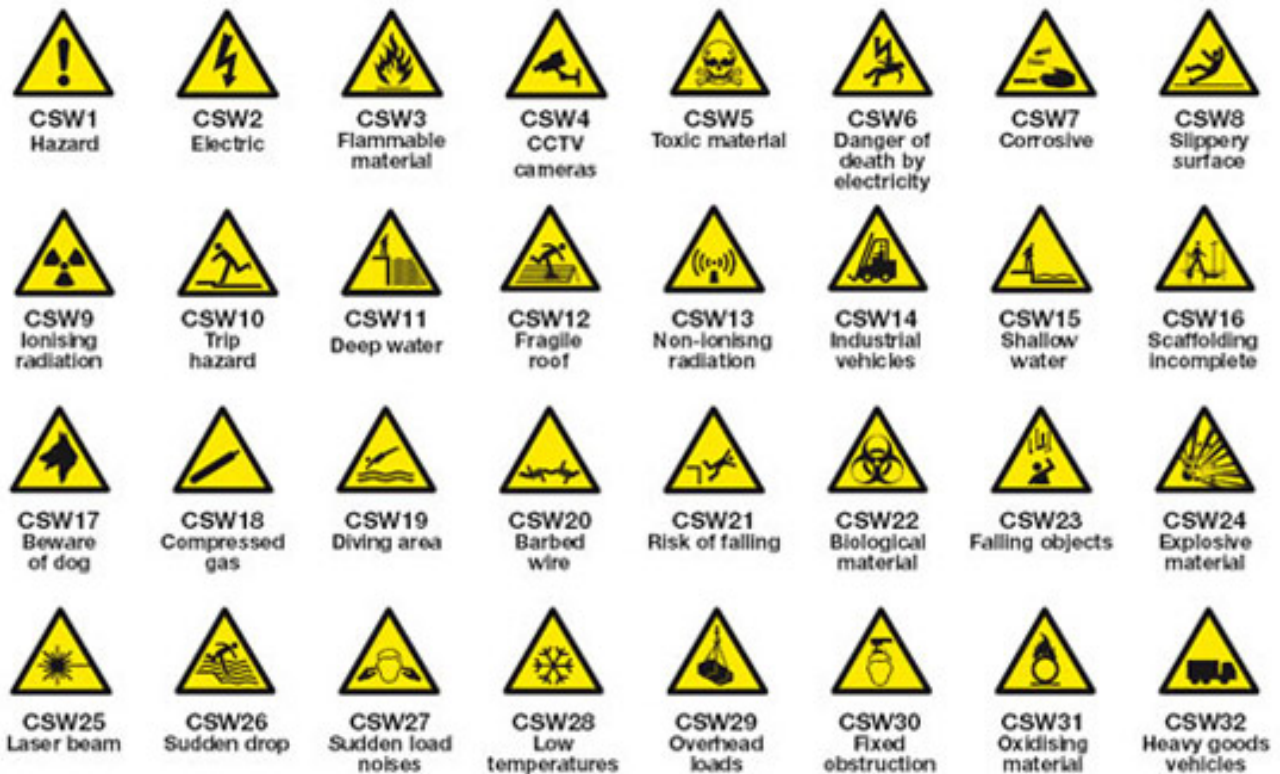
Figure 25.2: Typical safety signs at dry-docking site
