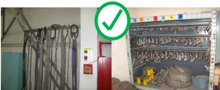
Figure 32.1: Storage of lifting accessories
