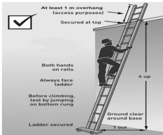
Figure 15.2: Correct set-up of ladder
