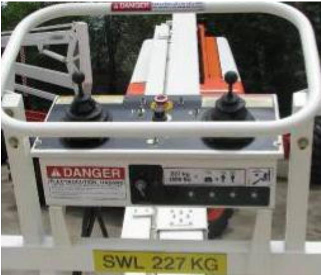
Figure 16.4: Checking safe working load (SWL)
