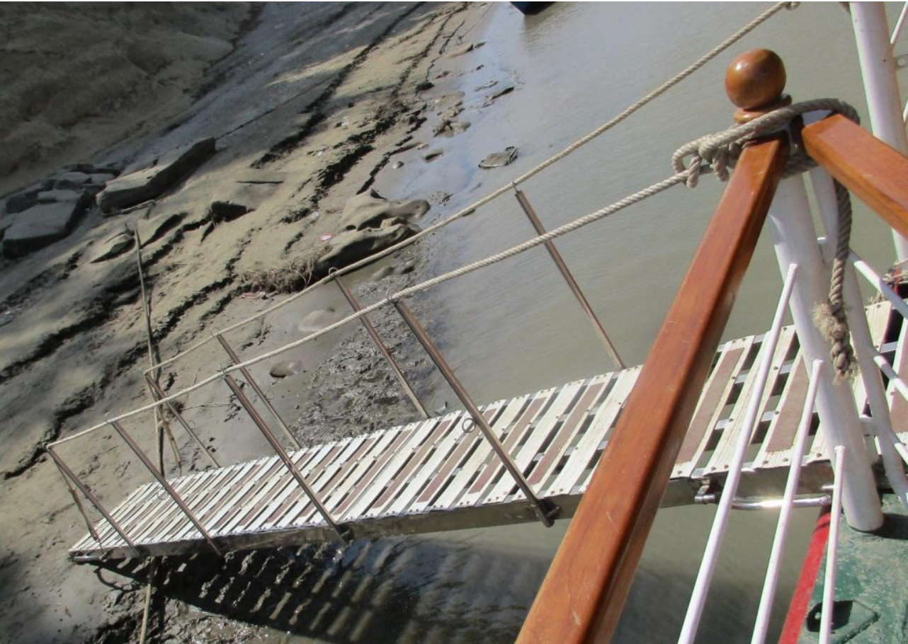
Example B: Gangway not manufactured by recognized national, or international standards, not properly secured and slope > 30 degrees.
