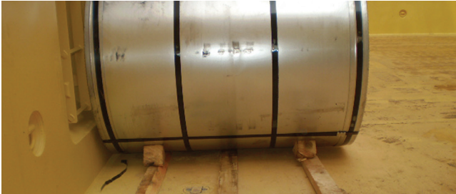
Figure 45: Coils wedged in position
