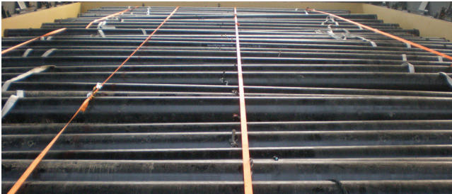
Figure 43: Pipes secured in the hold, but lashings are of little value
