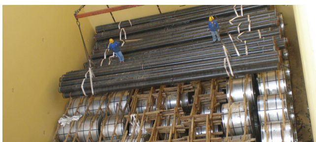
Figure 51: Pipes loaded on top of coils need to be securely lashed to prevent movement. Dunnage has been placed between the pipes and the longitudinal bulkhead
