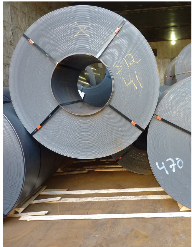
Figure 21: This key coil appears to exceed the 60% rule.
