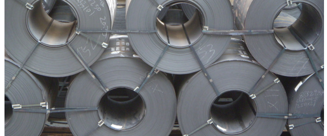
Figure 47: Coils stowed and lashed together with steel bands
