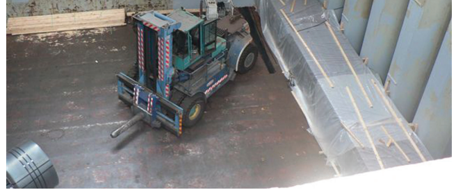
Figure 46: Coils being stowed by a forklift fitted with a single round tine
