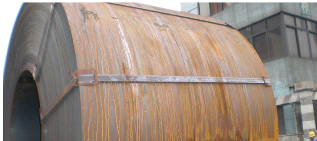
Figure 50: Condition of coils at discharge port – rusted
