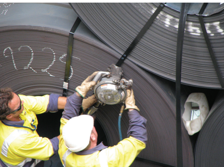
Figure 33: Steel bands are pneumatically tightened
