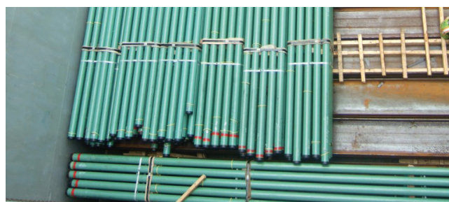
Figure 52: Pipes are stowed fore and aft, and athwartships. Dunnage has not been placed between the pipes stowed athwartships and the ship's side bulkhead
