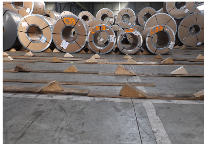
Figure 38: Coils prior to stowage correctly wedged
