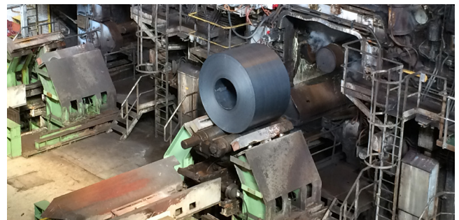
Figure 2: Hot rolled coil after rolling
