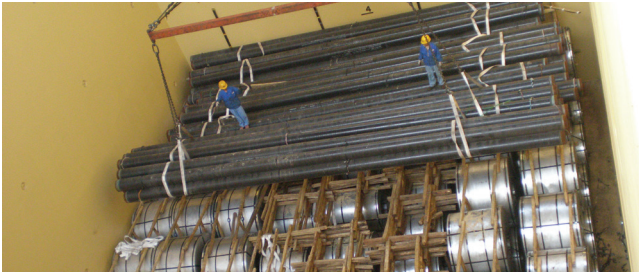
Figure 44: Pipes loaded on top of steel coils
