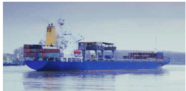
Figure 7: Typical arrangement for con-bulker with gantry crane
