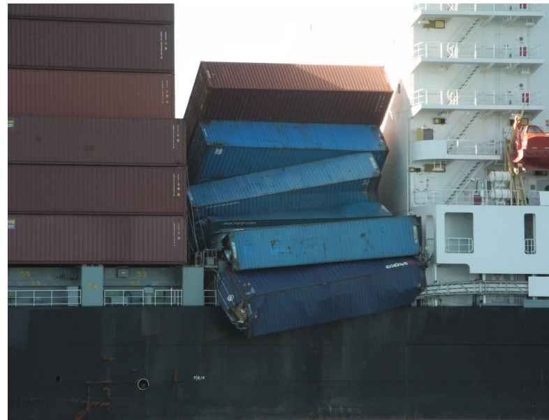
Figure 42: Outboard container damaged by adverse weather and incorrect stowage
