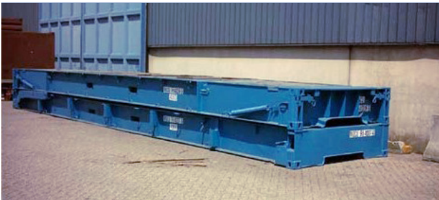
Figure 16: Two flat racks
