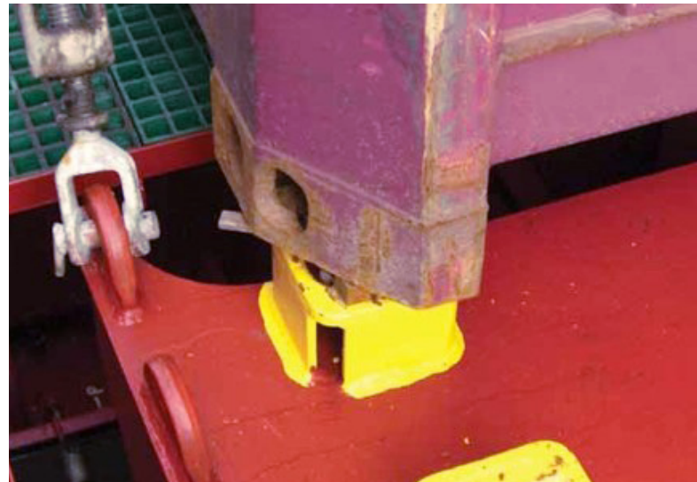
Figure 17: Corner casting arrangement for a Euro container
