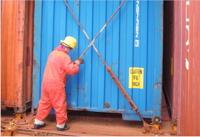
Figure 12: Do not lash to the overhanging end of a 45ft container
