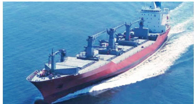
Figure 9: Multipurpose general cargo ship with the capacity to carry containers on deck
