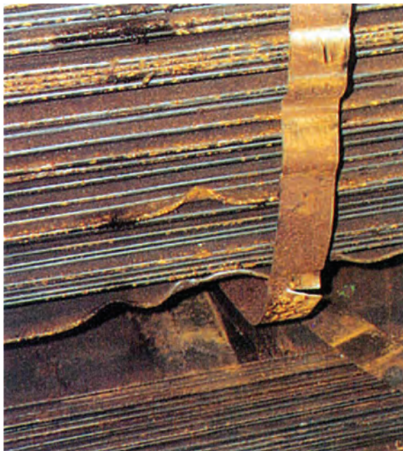
Fig. 25. (above) Bundle of stainless steel plates. Mechanical-damage clause: edges dented at centre where handling gear marked. Affects two plates
