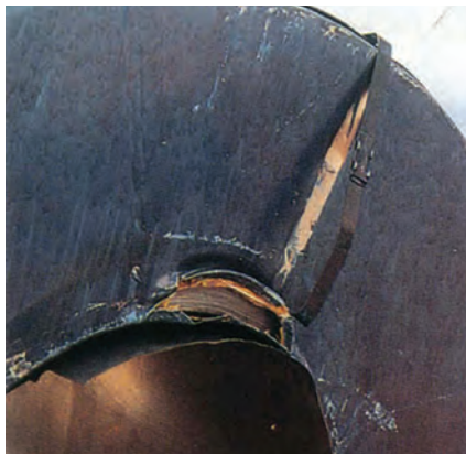
Fig. 18. Wrapped coil damaged by forklift. Mechanical-damage clause: packing torn open in one place at inner circumference. Visible cargo is scored. Affects 15 windings
