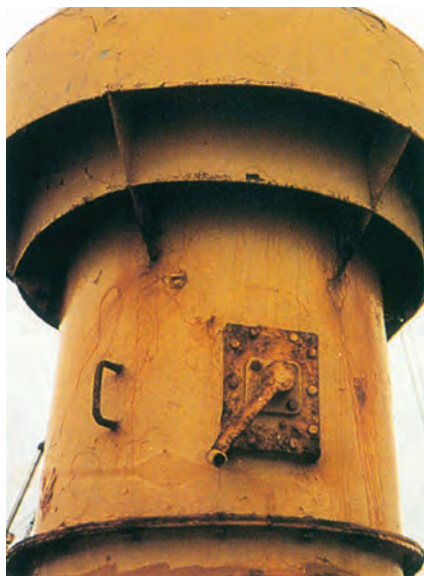
Fig. 31. Mushroom-headed natural-draft cargo-hold ventilator with handle-operated internal closing flap. The handle and flap should be checked and operated to ensure that full opening and closure is possible
