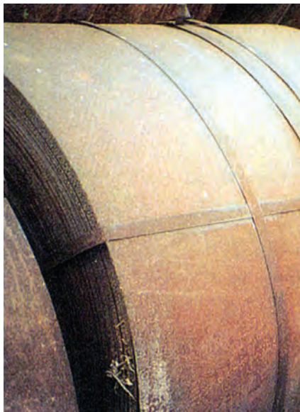
Fig. 8. Hot-rolled steel coils. Surface-condition clause: rusty
