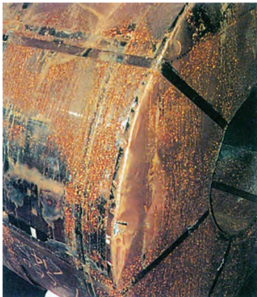
Fig. 14. Wrapped coil with streaky rust brought about by dripping water from 'cargo sweat'. Surface-condition clause: packing rust stained, streaky rust indicates previous contact with water
