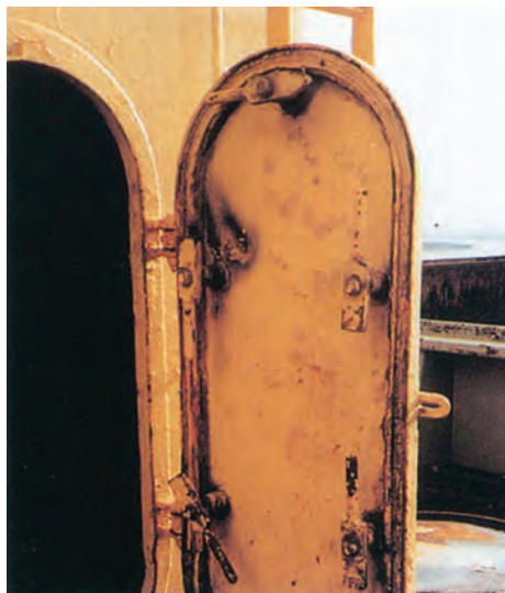
Fig. 29. Mast house door leading to a cargo hold internal escape hatch. Closer examination reveals that the door's sealing rubber has been painted over and is hardened, excessively compressed and perished leaving the cargo vulnerable
