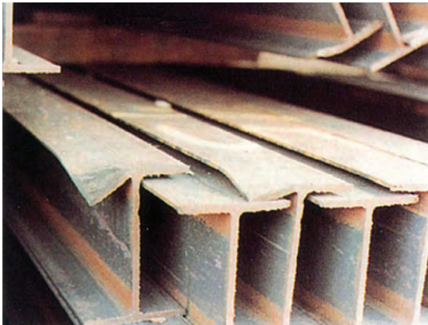
Fig. 24. (below) Nest of beams. Mechanical-damage clause (left hand beam): flange bent in one position at end
