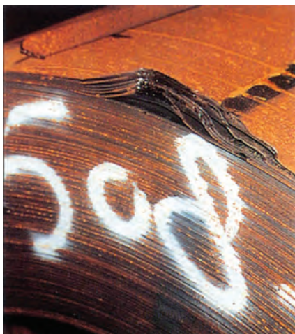
Fig. 21. Coil damaged by forklift. Mechanical-damage clause: edges buckled at outer circumference where handling gear marked. Affects six windings
