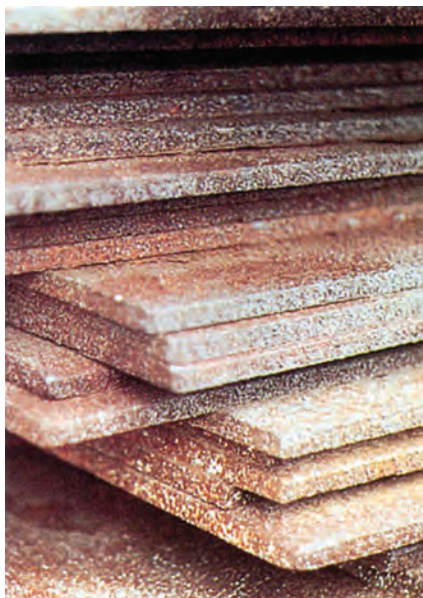
Fig. 10. Plates. Surface-condition clause: rust with pitting
