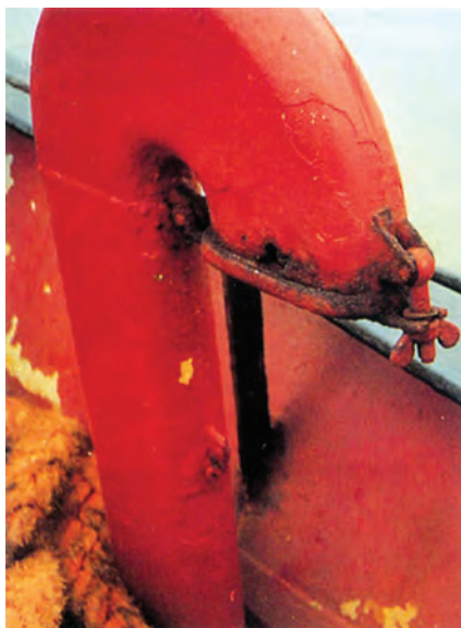
Fig. 30. A goose-neck air pipe with a closing flap secured by a wing nut. However; the pipe has rusted through above the flap and is no longer weathertight
