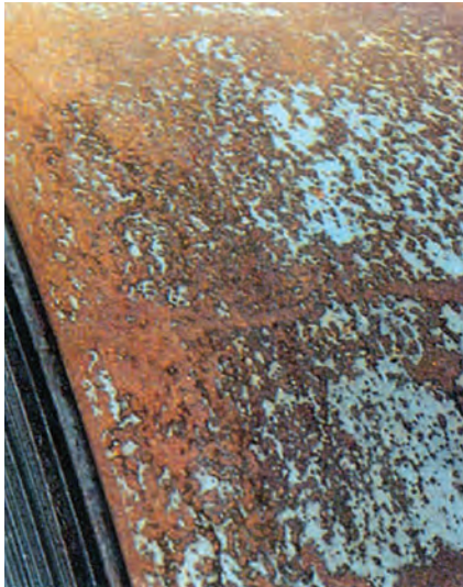
Fig. 11. Hot-rolled steel coil. Surface-condition clause: rust stained, rust spots apparent
