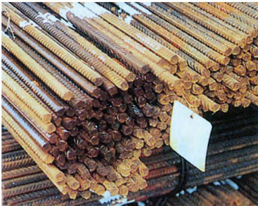
Fig. 4. Reinforcing bars in bundles with dampness evident. Surface-condition clause: rust stained, wet before shipment
