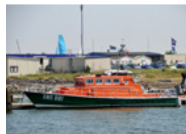
SNS 091" Ouistreham rescue boat: polyester L = 17.60 m - l = 4.20 m P = 2x279 Kw /Volvo TAMD 122A"
