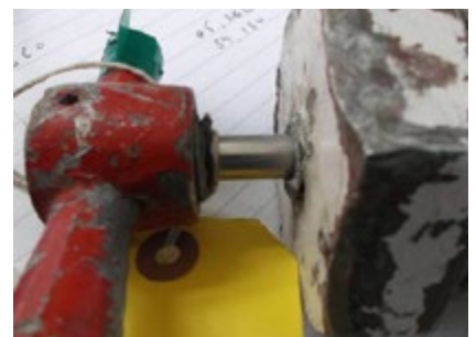
Figure 2 - Threaded element for lever & spindle sheared
