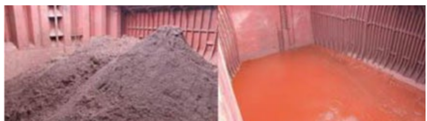
Iron ore fines before and after liquefaction.
