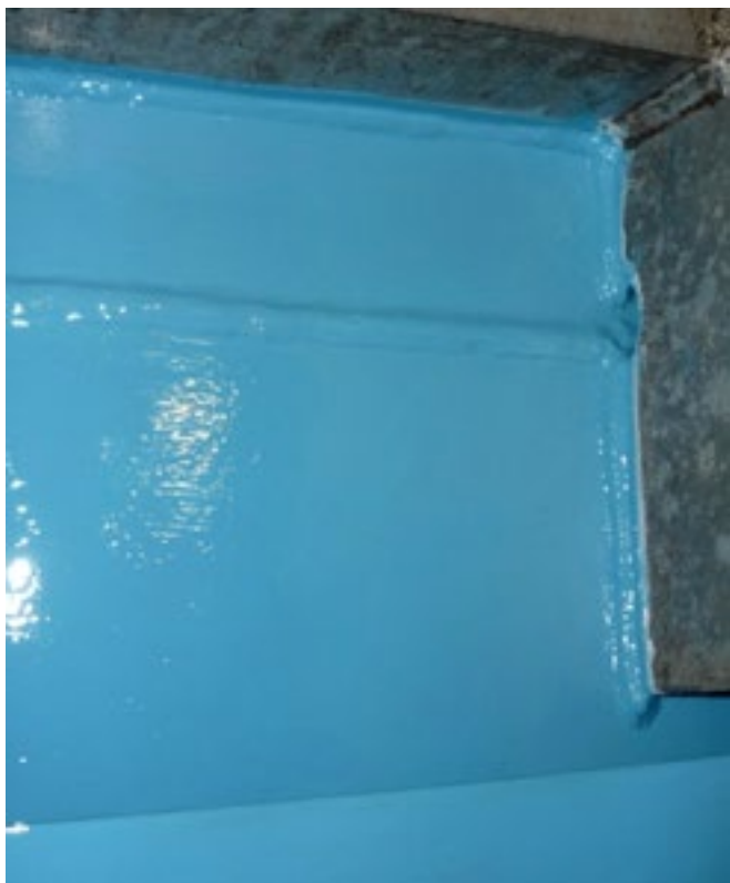
1030 Blue Coating protection in an integral aluminium fuel tank
